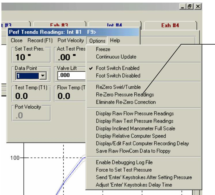
During testing, you can click on Options, then click on one or both of the “ReZero” options to better “fine tune” the factory calibration. Using a factory calibration from the numbers above and then using the “ReZero” options is generally sufficient for most testing.
