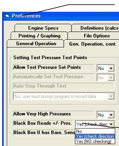
A Preference in the program lets you have the sensors measure both + and - pressure. This lets you simplify your bench design. Otherwise you need valves to keep the high pressure side always the high pressure side of the manometers and sensors, like in a Superflow bench, or swap hoses where you switch from Intake to Exhaust flow direction.
