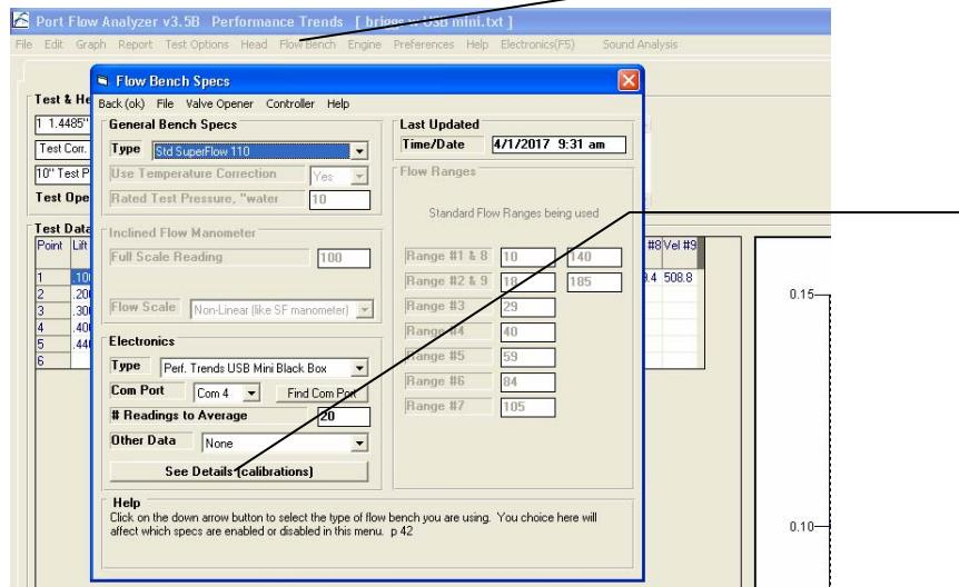
Click on Flow Bench at top of Main Screen to bring up Flow Bench specs screen shown here.
