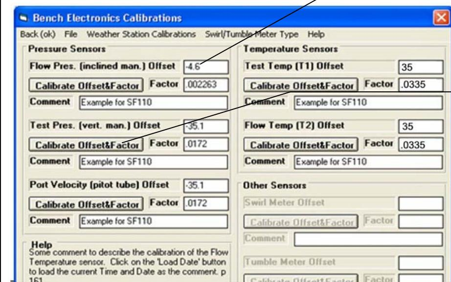
Click on See Details (calibrations) to enter typical calibrations for sensors in Mini USB.
