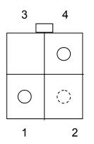
Pin numbers are visible from the back of the connector. When you wire up, make sure the pins match up with the sockets on connector on Blowby Logger harness.
