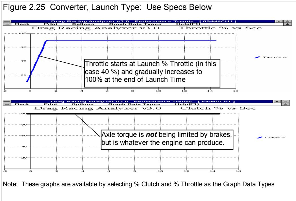
2. At the start, the brakes are released and the throttle is opened as specified by the Launch % Throttle. The % Throttle is gradually increased from the starting percents so it is at 100% at the end of the Launch Time.
