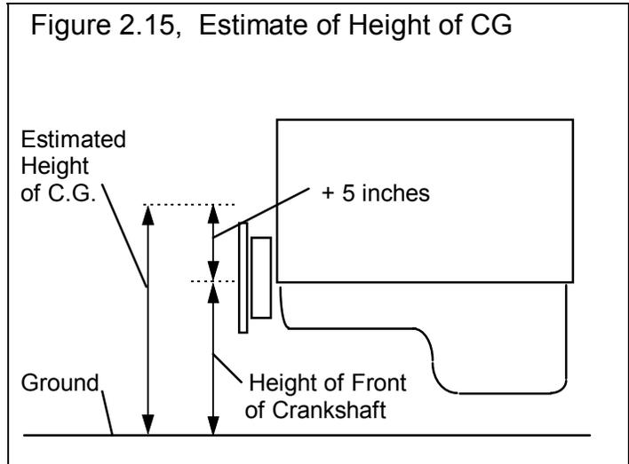
Estimate the Height of CG of motorcycles as half way between the rider's shoulders and the engine's crankshaft. For example, if the height of the rider's shoulders is 40" and the crankshaft centerline is 14", the Height of CG would be  $(40 + 14) / 2 = 27"$ . Obviously, driver position has a significant effect on this parameter.
