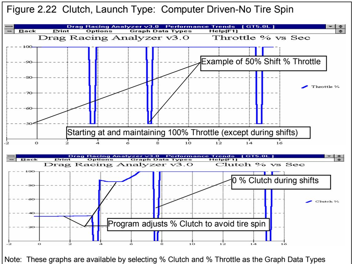
3. When the engine and clutch RPM both reach the 1-2 Shift RPM (no clutch slip), the clutch is disengaged, the throttle is
