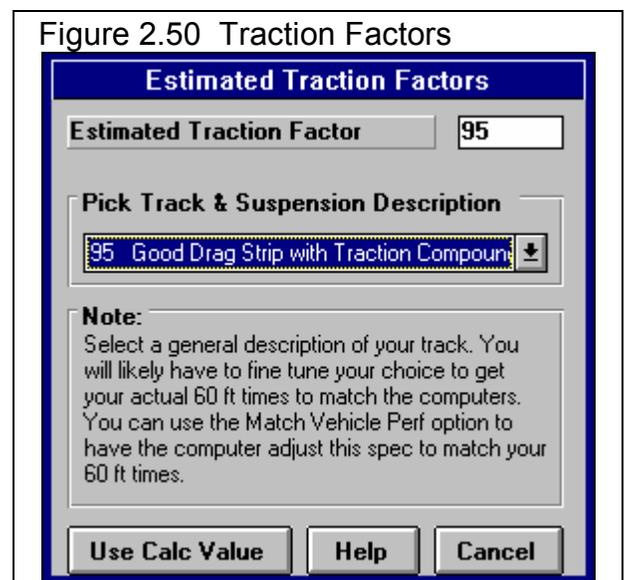
The Traction Factors in this list are very general. You will probably have to fine tune this spec based on your vehicle's actual 60 ft times. The program can also determine Traction Factor with the Match Vehicle Performance command at the Main Menu.
