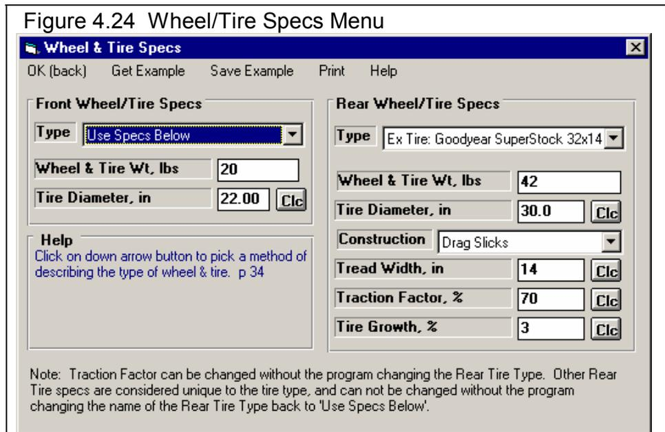
For Rear Wheel/Tire Specs, select Pick Example Wheel/Tires from the list of Types. Select the Example Goodyear Superstock 32 x 14 Drag Slicks. The Wheel & Tire specs menu should now look like Figure 4.24.
