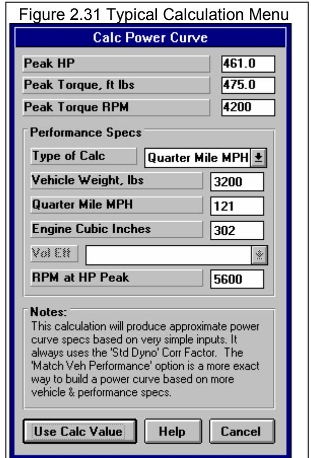
You would be ready to Use Calc Values if the RPM at Peak HP was correct. From reading in this section, you see that a good estimate of RPM at Peak HP is about 500 RPM less than the RPM you shift at or go through the traps at. So you decide to adjust that up to 5500 RPM. You see Peak HP stay the same but Peak Torque and Peak Torque RPM updated to new, more accurate readings.
