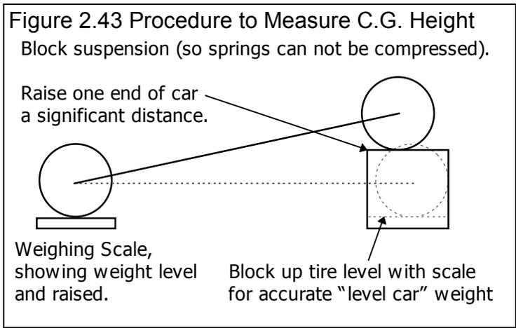
Raising a typical car about 20 inches (quite a lot) will only show a weight increase of 30-60 lbs for most cars. Therefore, this process requires very precise weight measurements. Some tips to improve the accuracy of the procedure include:
