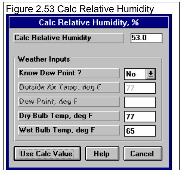
Relative humidity or dew point can be manually read off a Psychometric chart from these two readings. This calculation replaces reading the chart. The Wet Bulb Temp must be less than the Dry Bulb Temp.
