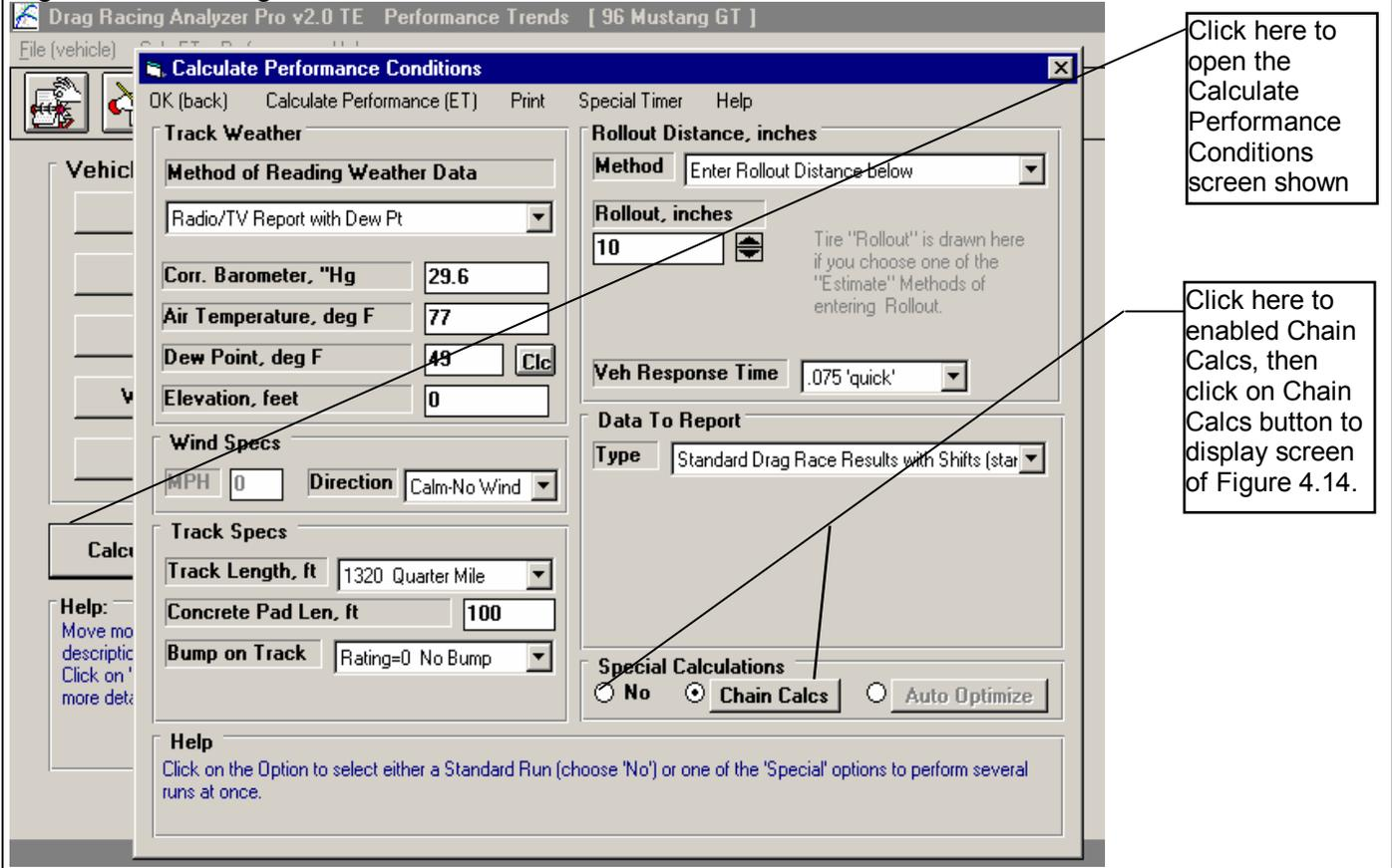
Figure 4.14 Chain Calculations Screen Setup to Try 7 Axle Ratios
