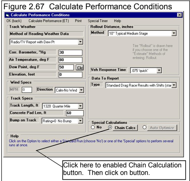
Figure 2.68 Chain Calculation Screen
