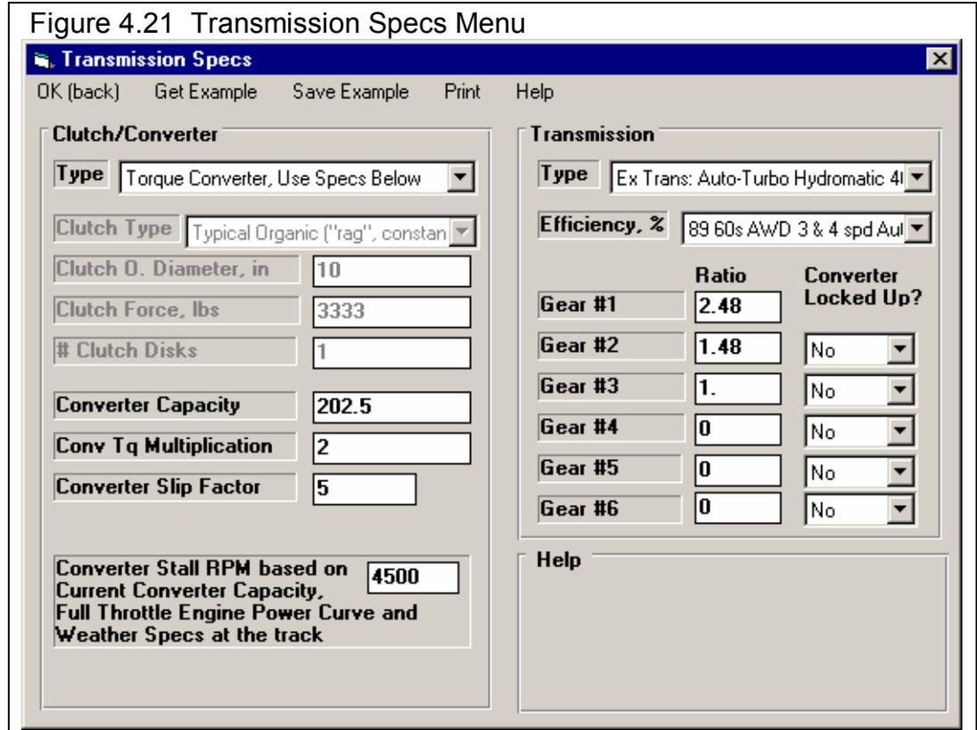
Figure 4.21 Transmission Specs Menu
