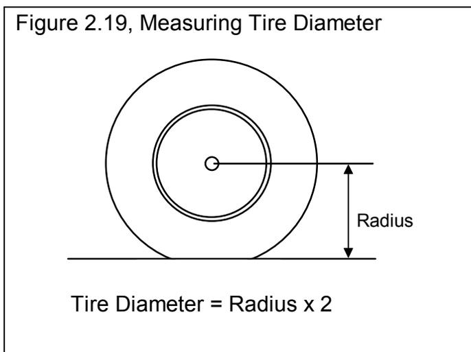
Since tires can squat as they are mounted on the car or as you change air pressure, a better estimate of the diameter is to measure the distance in inches from the center of the tire to the ground, while the tire is mounted on the car. This will give the radius, which you can then multiply by 2 to obtain your best estimate of the tire's diameter when mounted on the car.
