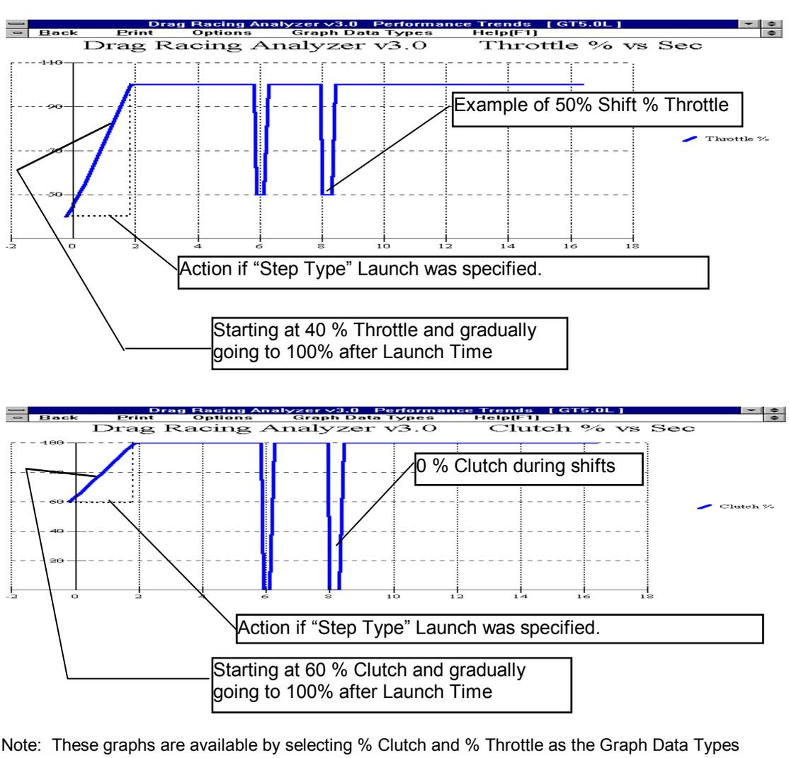
3. When the engine and clutch RPM both reach the 1-2 Shift RPM, the clutch is disengaged, the throttle is opened as specified by the Shift % Throttle, the gears are changed from 1st to 2nd, and when time has passed as specified by the Shift Time, the clutch is released 100% and the throttle is opened 100%.
