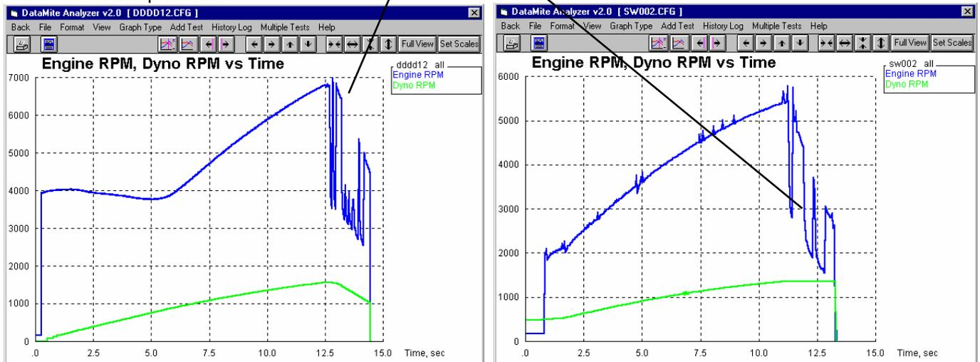
If the inductive pickup signal is too strong (you wrap the spark plug wire too many times), you may not be able to record Engine RPM at high RPM. Engine RPM may drop in half or all the way to 0 RPM.
