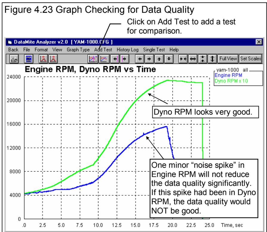
Now add the test you want to compare this test to by clicking on Add Test in the Graph Screen. See Figure 4.23. You will obtain a screen similar to Figure 4.21 on the previous page. Select the YAM-975.CFG test, which had a 9 3/4 inch exhaust flex. You should now obtain a screen similar to that shown in Figure 4.24. The YAM-975 has nothing that looks like a noise spike, so its data quality looks very good.
