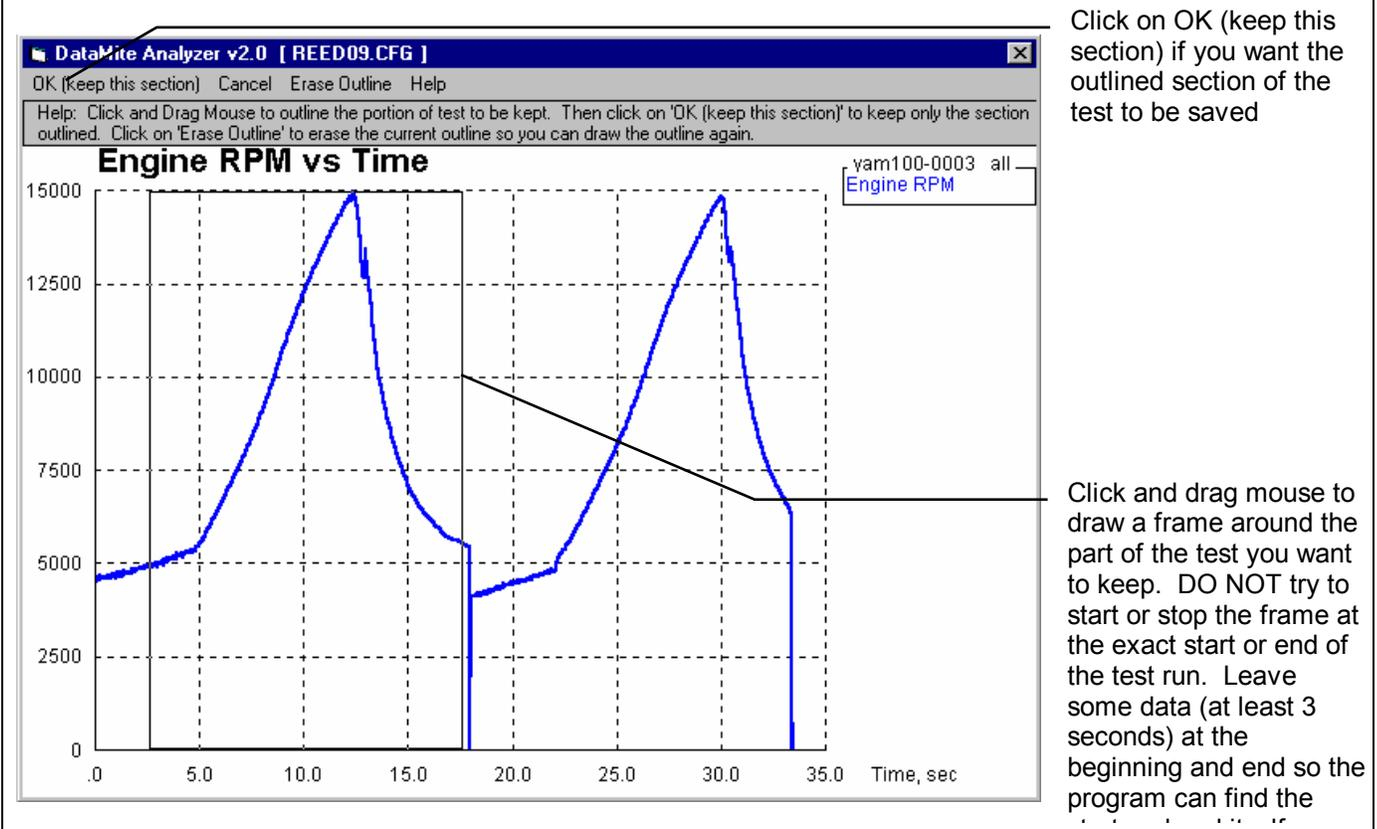
If you click on Edit, then Delete Beginning or End of File, you will be presented with a graph screen showing Engine RPM for the this entire test. Click and drag the mouse to draw a square frame around the portion of the test you *want to keep*. The rest of the test will be deleted. When you are satisfied with the section you've drawn, click on OK (keep this section) to be presented with the options shown in Figure 2.43.
