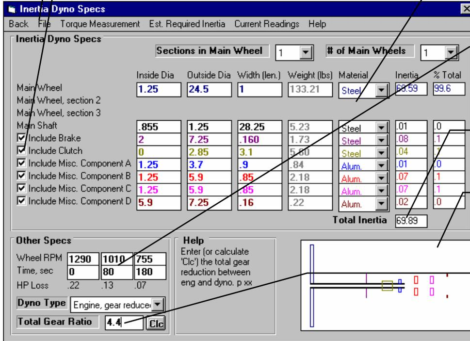
These numbers based on coastdown tests determine frictional losses in the dyno system for more accurate torque and HP numbers.
