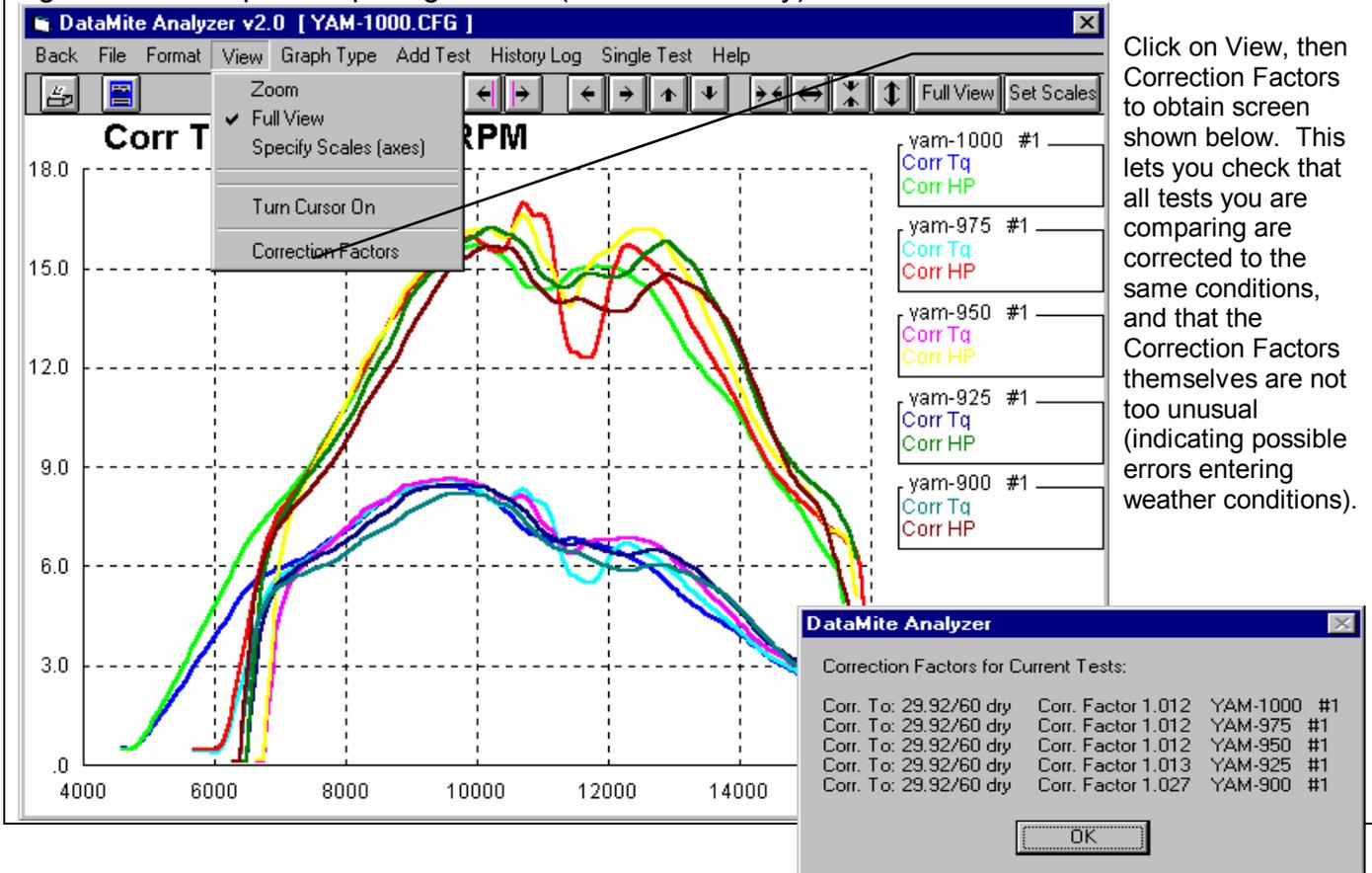
Click on View, then Correction Factors to obtain screen shown below. This lets you check that all tests you are comparing are corrected to the same conditions, and that the Correction Factors themselves are not too unusual (indicating possible errors entering weather conditions).
