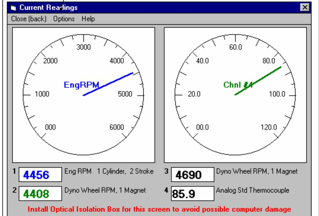
**IMPORTANT:** It is strongly recommended that you purchase Performance Trends Optical Isolation box if you use this screen while dyno testing an engine. This will prevent 'voltage spikes' from the engine passing back through the DataMite to your computer, possibly damaging the computer.
