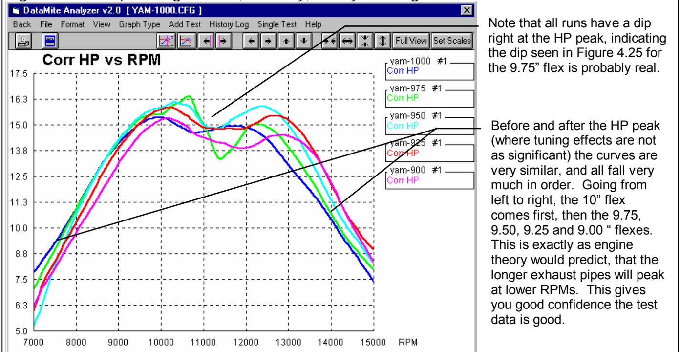
Note that all runs have a dip right at the HP peak, indicating the dip seen in Figure 4.25 for the 9.75" flex is probably real.
