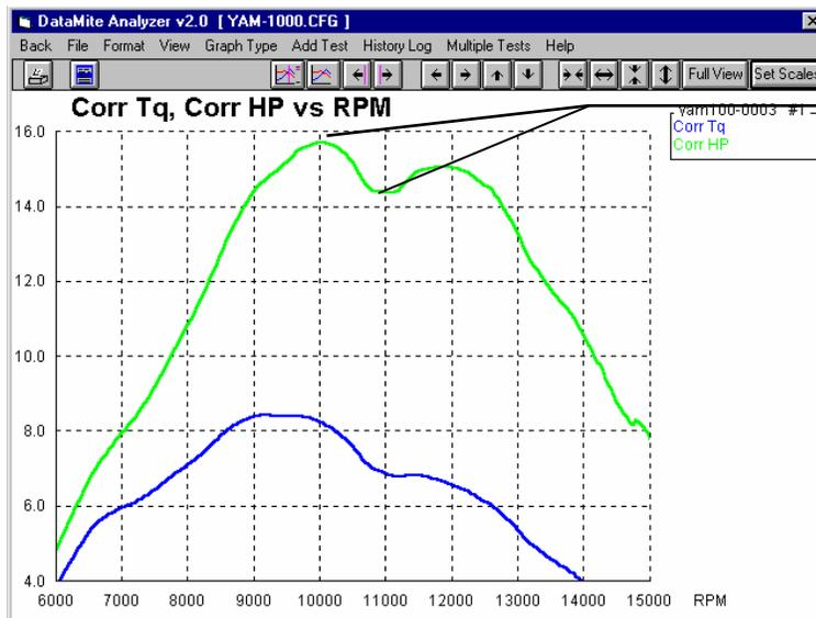
In most cases for torque and HP graphs, Filtering = Some is the best choice. The peak torque and HP values for this graph are fairly accurate and repeatable. For other types of data Some or None is best. Picking a Filtering Level too high can distort the data and cover up problems with the data.
