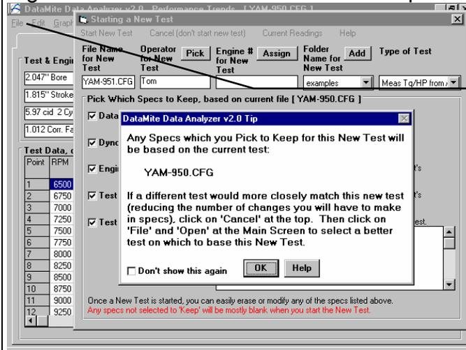
Click on File, then New (get data from DataMite) to bring up the New Test Screen.
