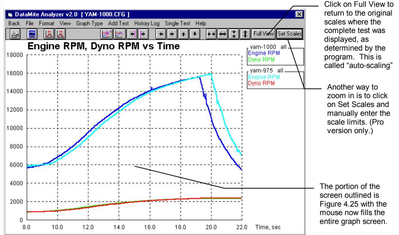
Figure 4.27 Time Aligning Two Time Graphs
