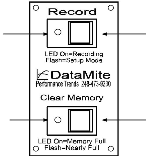
Setup Mode starts with displaying channel #1, engine RPM. Push Record button to Channel #2, and again to display Channel #3, etc.
