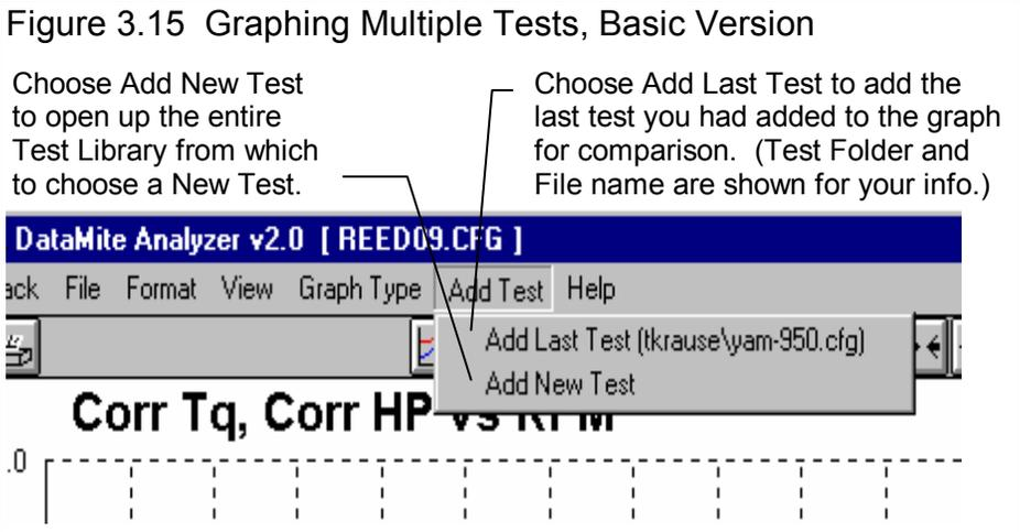
In the Basic version, you can only compare 1 additional test to the Current Test. If an additional test is graphed for comparison, the *Add Test* command changes to *Remove Test*. You must first click on Remove Test before the Add Test command reappears so you can add a different test.
