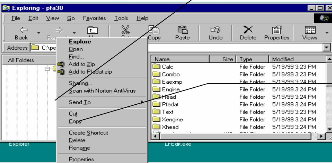
Right click (with the right mouse button) on the DTMDATA folder (not seen here) to open a menu of options.
