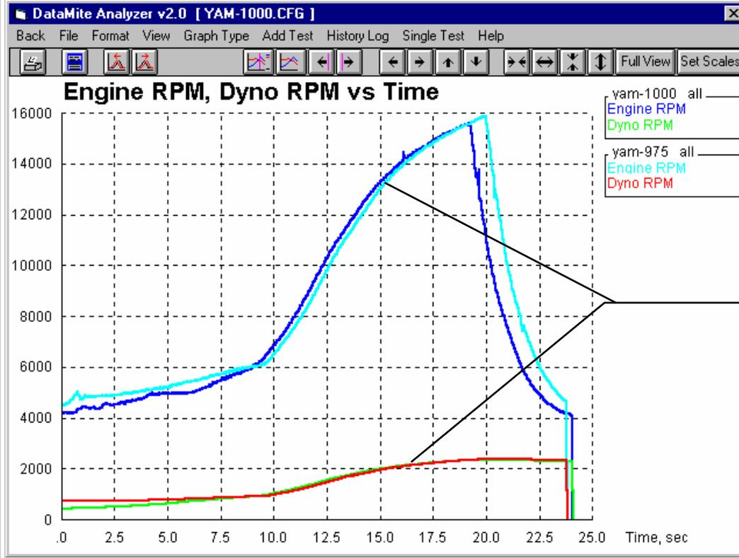
Note that in this graph the program decided NOT to multiply Dyno RPM by 10 as it did in Figure 4.23. Therefore, dyno RPM looks much smaller compared to Engine RPM in this graph.
