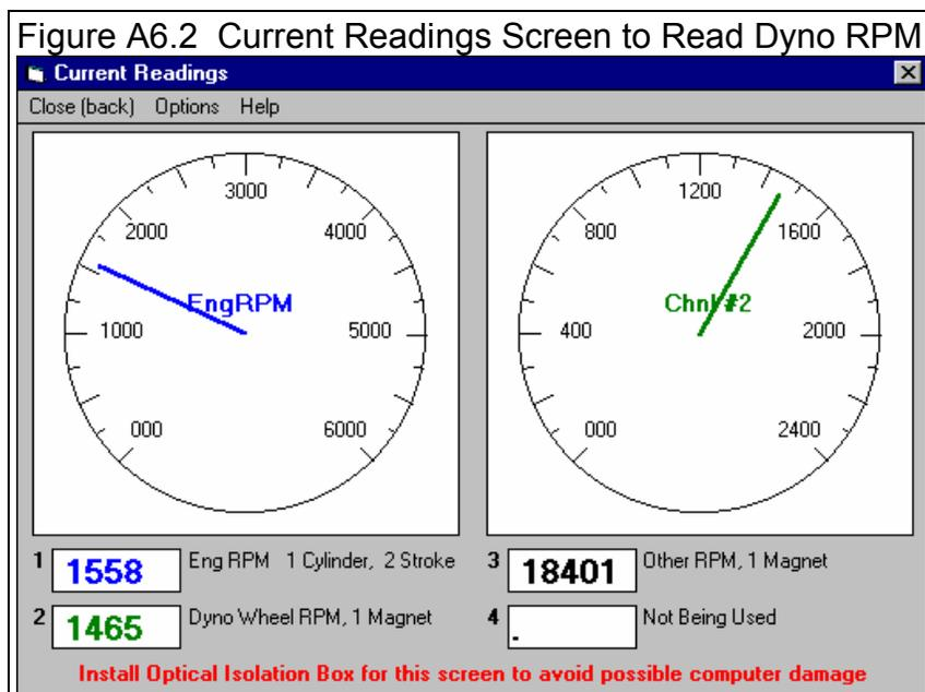
8. Stop the stopwatch at some RPM which is about 1/2 to 1/3rd of the RPM at which you started. Lets say this was 755 RPM at 180 seconds, that is 180 seconds after you started the stopwatch at 1290 RPM.
