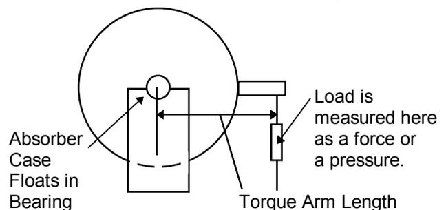
If this is your type of dyno, choose Torque Arm as the Torque Measurement type. The dyno screen now becomes very simple as shown in Figure 2.24. See Appendix 5 for calibrating a Torque Arm type of dyno.
