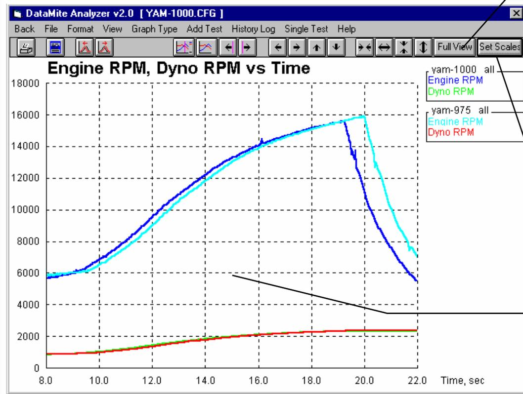
Click on Full View to return to the original scales where the complete test was displayed, as determined by the program. This is called "auto-scaling"
