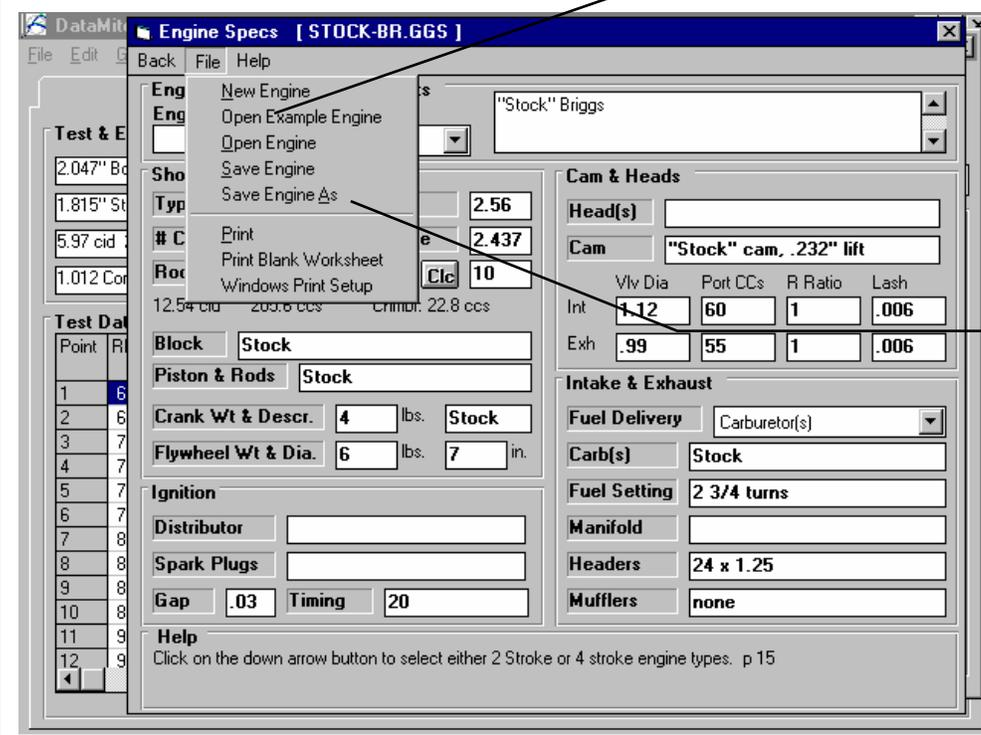
Click on File, then Open Example Engine to see if there are some Briggs specs saved as an Example Engine File. There are, so choose the STOCK-BR.GGS engine file to fill in much of this screen. Then you can go through each specs to make sure it matches your engine.
