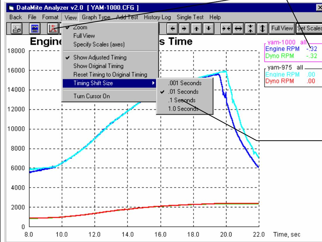
Click on these Time Align buttons to shift one of the tests over another. The amount of shift is shown in the legend. The test with the 10" flex had to be shifted back .32 seconds for good alignment with the 9.75" test. (One button is hidden by the "View" drop down menu.)
