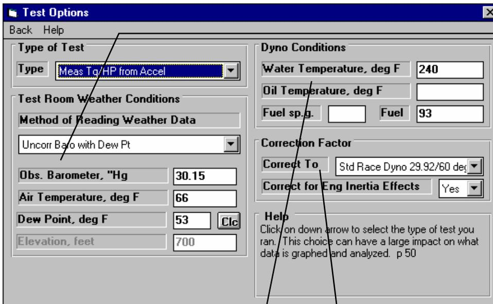
If you are going to compare and analyze Corrected torque and HP, then it is critical you enter accurate weather conditions for each test. Assume you have a portable weather station in your shop which gives Barometer in inches of Mercury and dew point. For best accuracy, the air temperature you enter should be the temperature right before the air cleaner or carb. However, be sure the temp sensor is not getting wet from fuel "stand off" from the carb.
