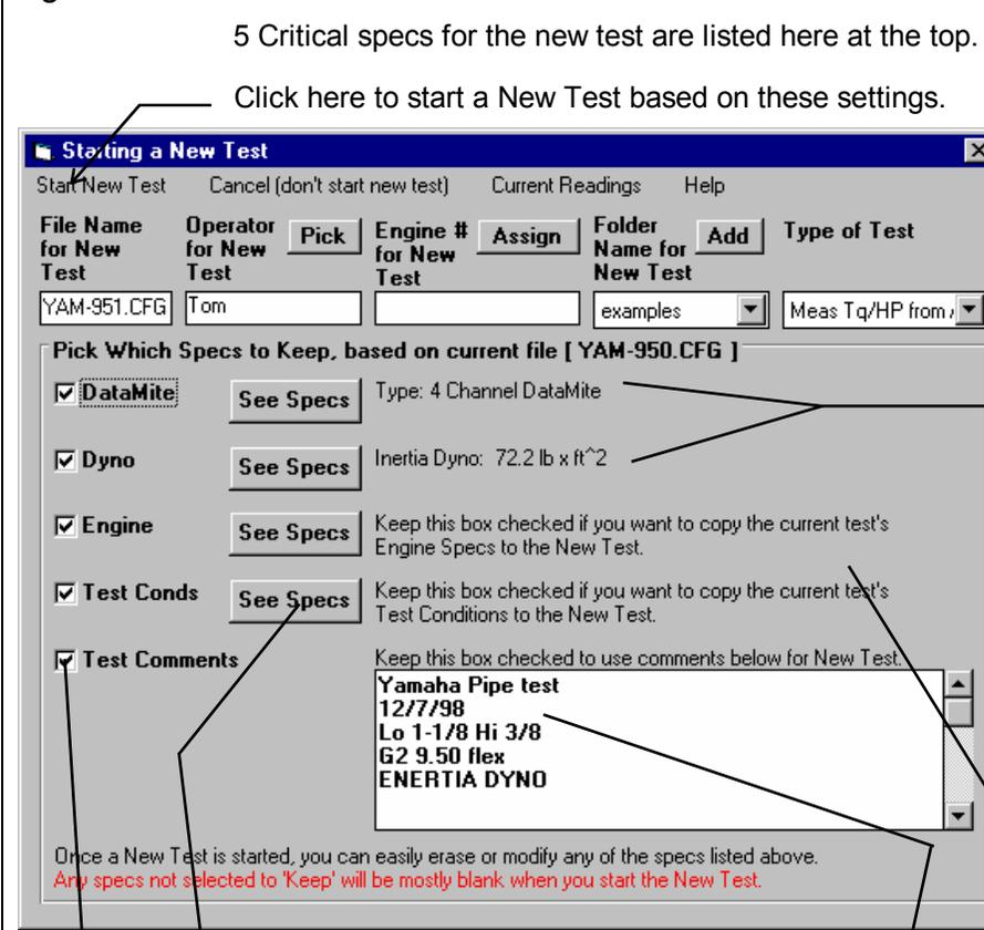
If this is the first time you have started a New Test and you haven't set up any Master Dyno or DataMite specs, the preview will say no Master Specs. You will have to fill out these specs before you can start the New Test.
