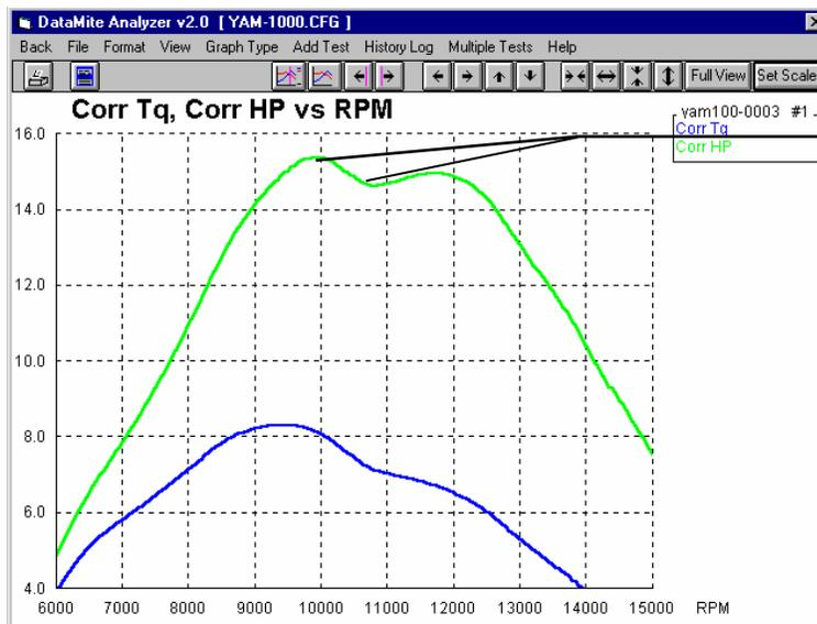
Note that the peak is the lowest and the valley is the least deep when filtering is the most, in this case Heavy. Heavy Filtering can hide problems with data. Before you use Heavy Filtering, be sure to check the data with Filtering set to None first.
