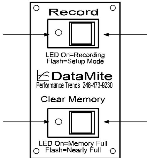
Push Record button to pause recording data (Record LED goes Off). Push Record button again to resume data recording (Record LED comes back On).
