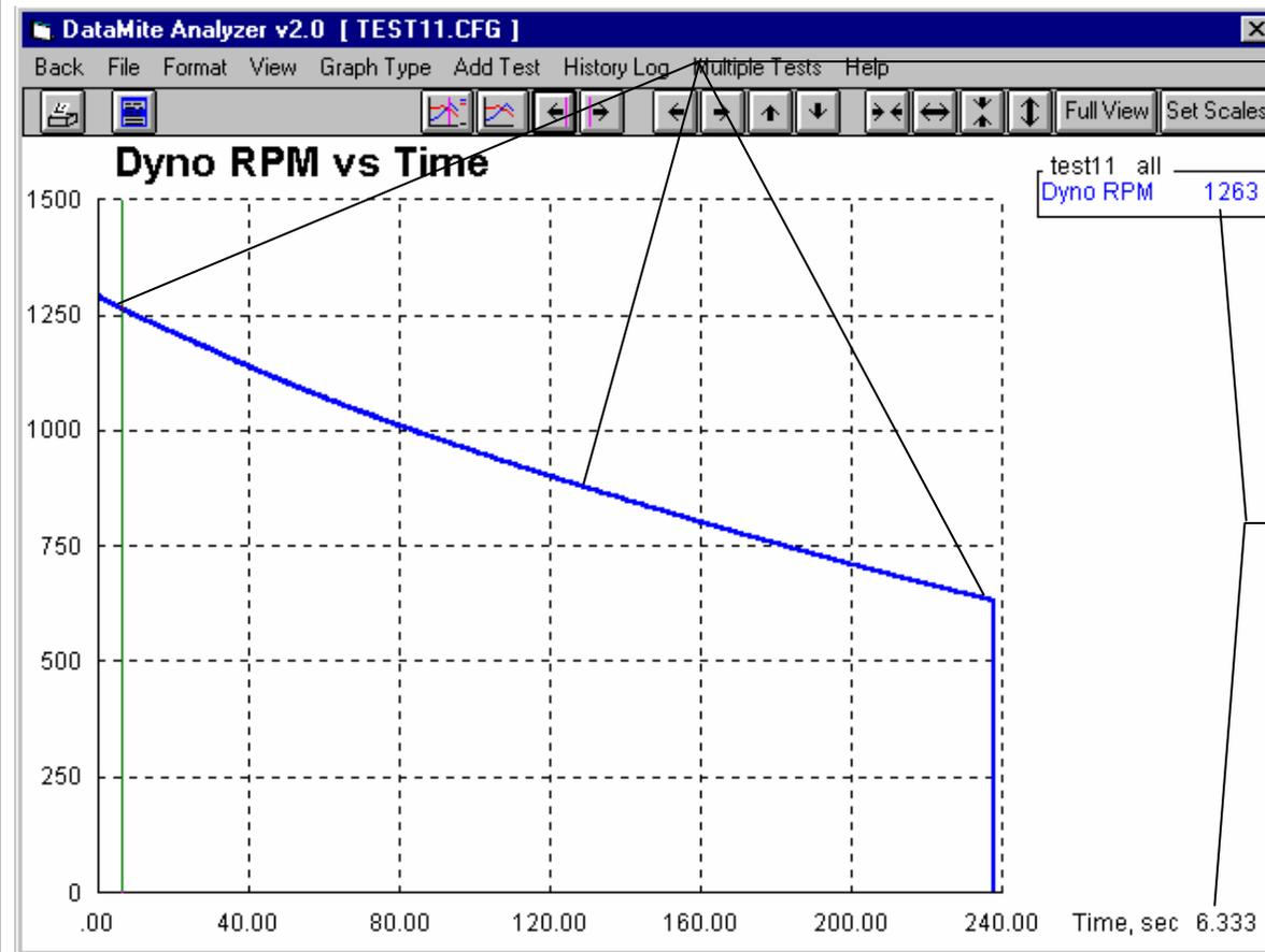
Use the cursor to find the Dyno RPM at 3 different times during the coastdown. These times and RPMs should be spread out as much as possible.
