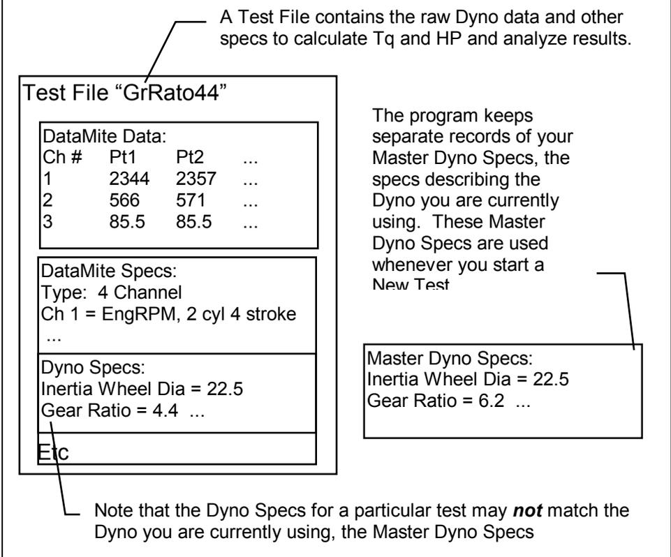
Figure 2.20 Dyno Specs Menu for Inertia Dyno (Pro Version)
