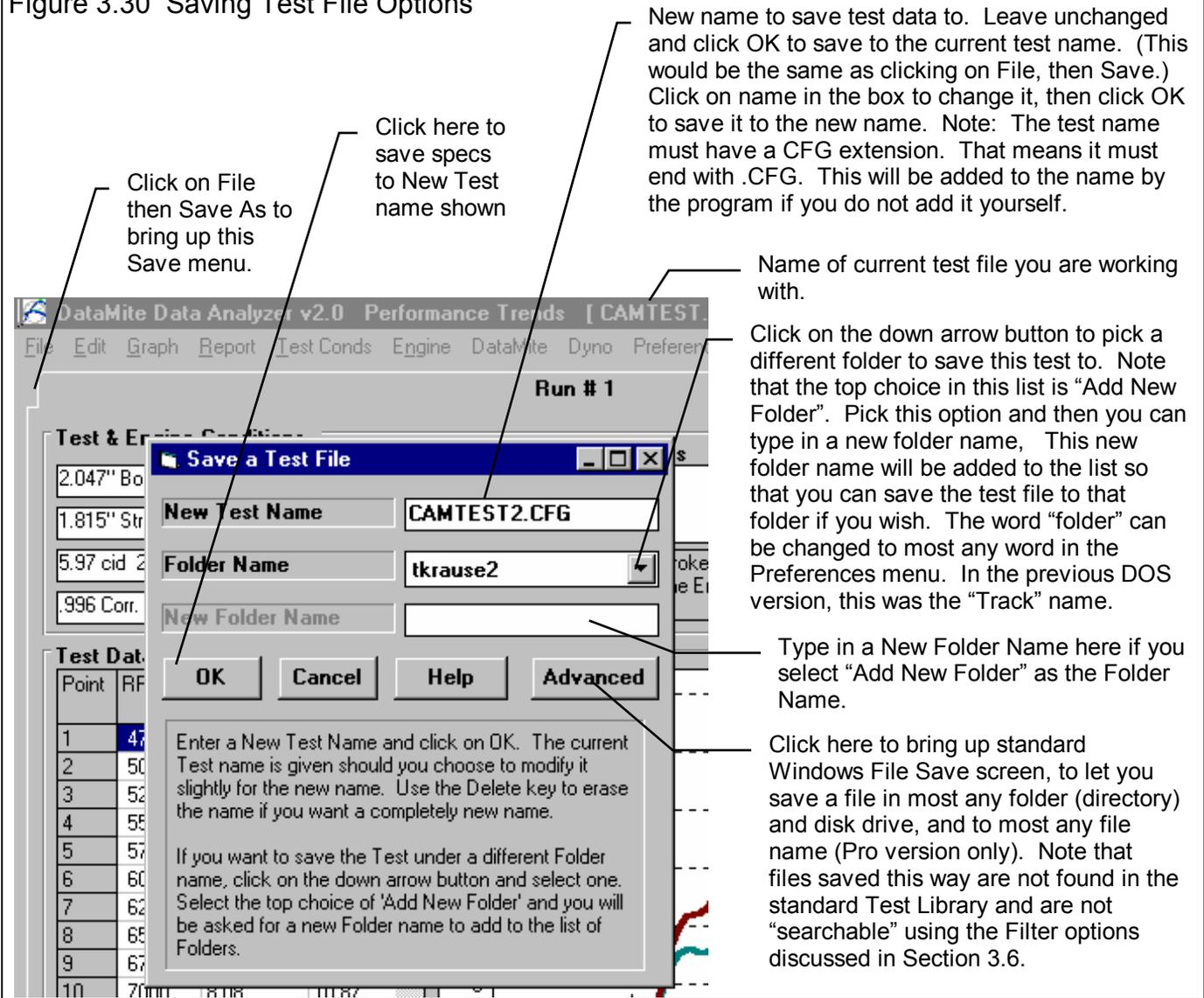
To save a Test File, you will be presented with the Save Window as shown above. The program suggests a new test name which is the same as the current test name shown at the top of the Main Screen. If you want to save your changes to the same name, simply click on OK. This will update the current test file with your latest changes.
