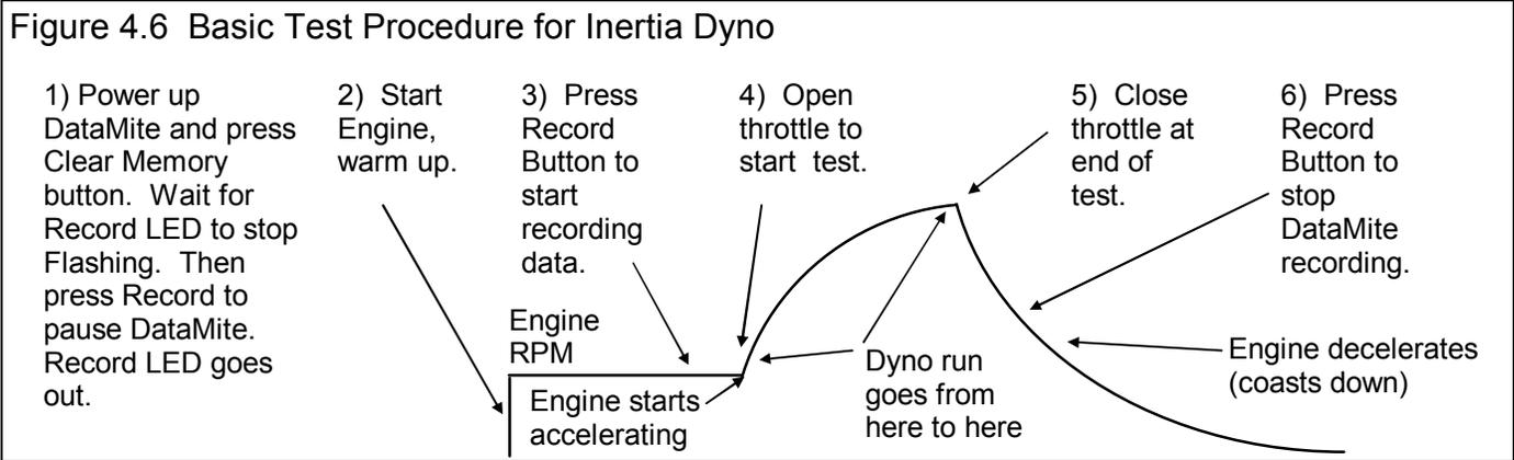
1. Power up the DataMite. When the LED by the yellow Record button stops flashing, press the red Clear Memory button to erase the DataMite's memory. Then when the LED by the yellow Record button comes on steady (stops flashing), press the yellow Record button to pause the DataMite (stop its recording). The Record LED will go out. You could omit the step of pressing the Clear Memory button which would keep any data already recorded by the DataMite, but this would not be recommended for beginners.
