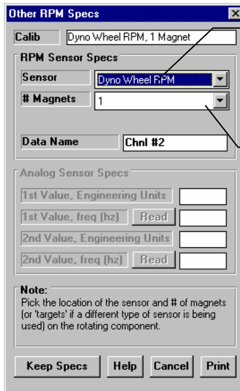
Pick Dyno RPM for channel 2 and Other RPM for channel 3. You would open this menu twice, once for each channel you want to change.
