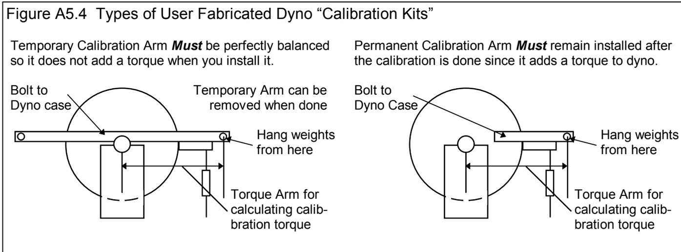
The permanent Calibration Arm method of Figure A5.4 is more accurate as you don’t have to be so exact about the balance of the calibration arm. If you choose that method, be sure the arm does not stick out so much you keep banging your knee into it!
