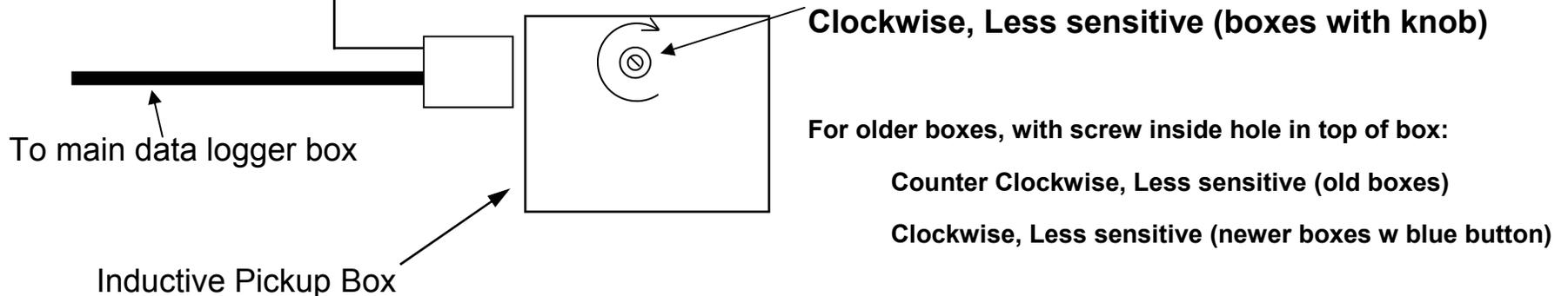
The **BB2-IPUP** replaces the Inductive Pickup Box shown above. This connector plugs into same harness connector as where the Inductive Pickup Box would plug into.
