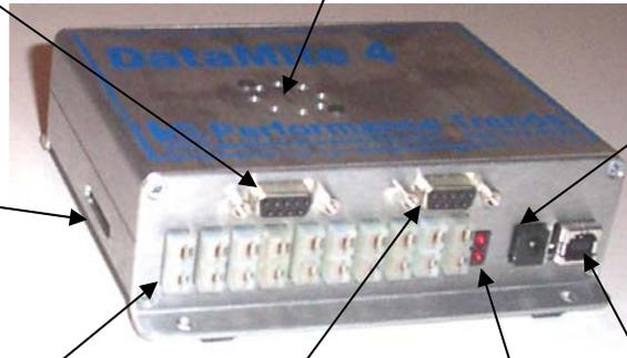
**GPS Connector** Is used for the GPS sensor and for 0-5 volt analog outputs. \*\*\*
