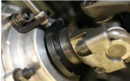
Use Loctite or RTV on all threads to prevent them from backing out.
