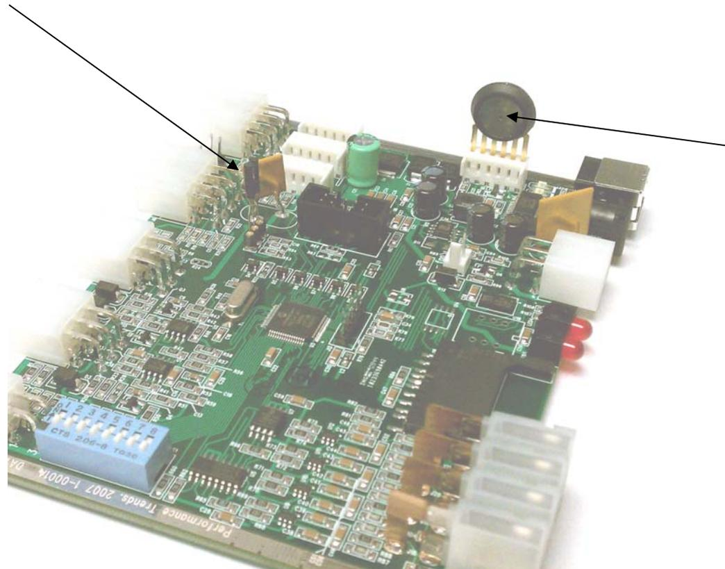
Barometer sensor, with metal side facing in toward center of board.
