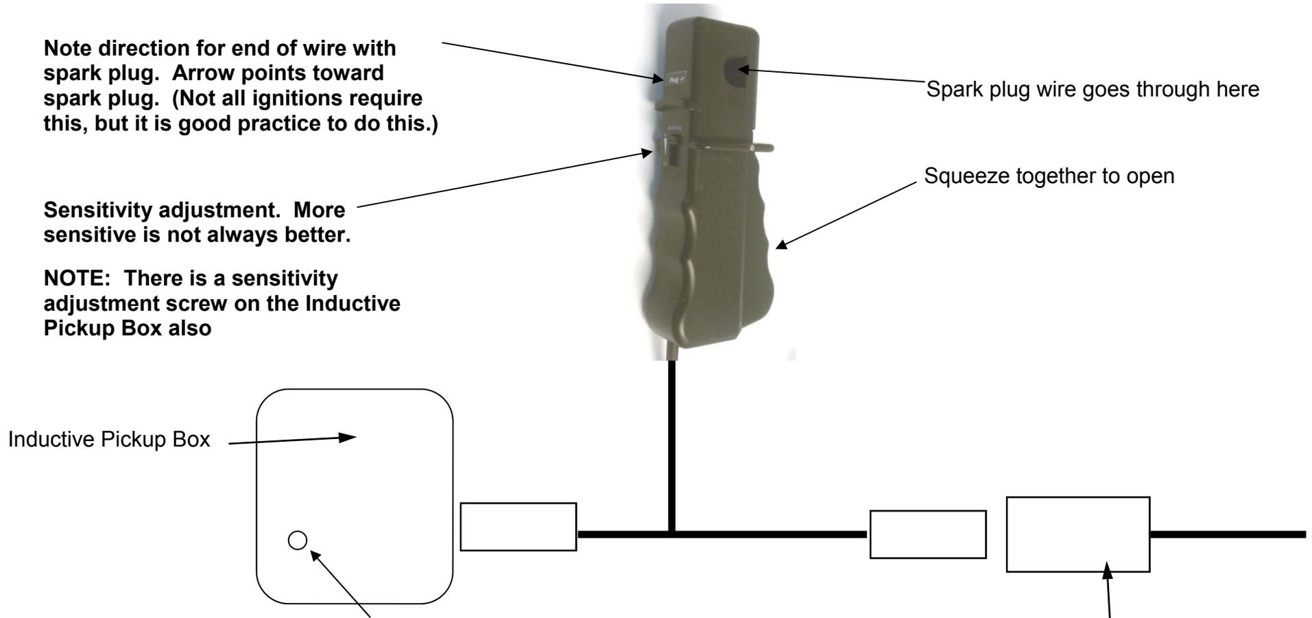
**Sensitivity Adjustment: Counter Clockwise, Less sensitive** DO NOT let metal screwdriver slip off screw or you risk shorting out the board inside. Box typically comes from factory with sensitivity set to maximum sensitivity. This is a 15 turn pot, so you can make several turns and still have adjustment. When it gets to either end of adjustment, it just slips (you may feel it click) to avoid damage.
