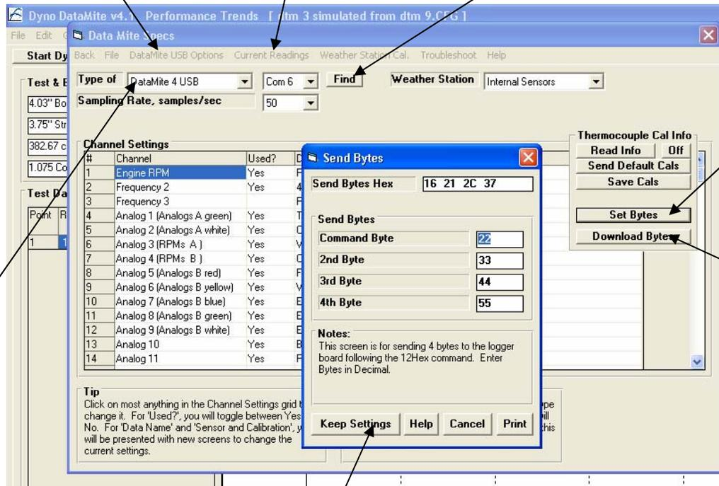
7) Click Download Bytes to send bytes in proper command string and CRC to logger board.
