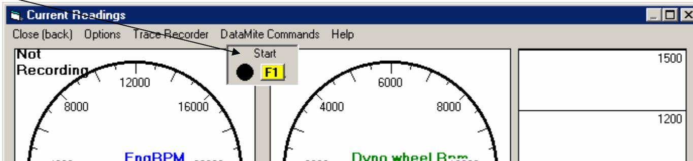
**IMPORTANT:** If you do not have the switch plugged into the correct channel, recording may start automatically as soon as you go to the Current Readings screen.
