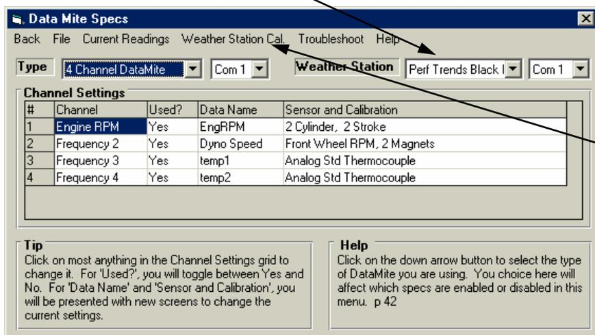
Click on Weather Station Cal. (visible only after you select ‘Black Box’ as the weather station) to bring up the calibration screen shown to the right.
