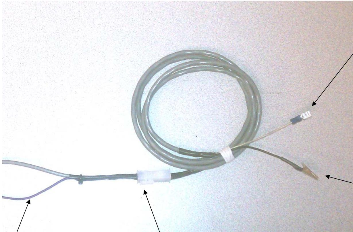
Spade connector for Tach Out, Spark Out, or similar "tach" signal from MSD or similar engine controller or negative side of coil.
