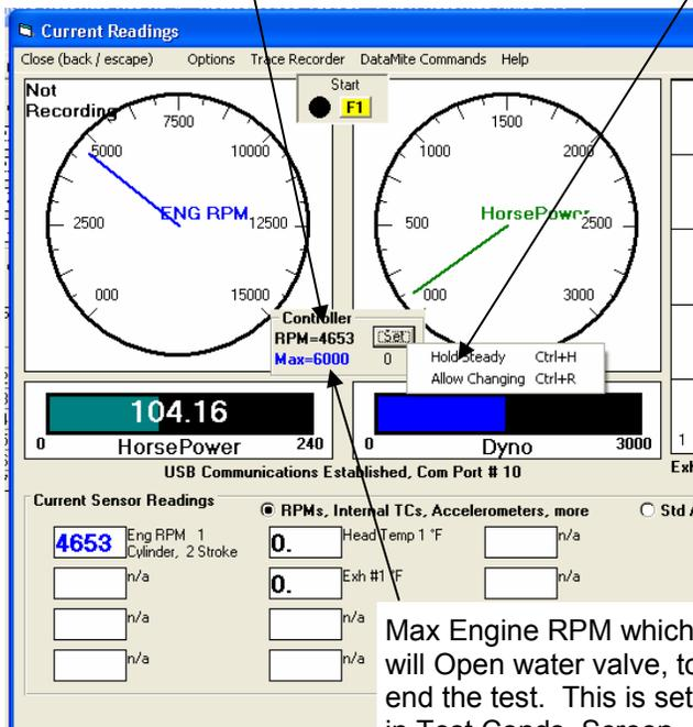
Max Engine RPM which will Open water valve, to end the test. This is set in Test Conds. Screen, shown to left.
