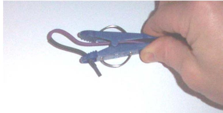
3) Finished clip installation should look as it does below. The clip is only to provide a convenient way to attach the purple wire to your plug wire. To adjust sensitivity, you need to adjust the sensitivity screw in the inductive pickup box. (Older inductive pickup boxes did not have this adjustment) Sometimes you may want to remove this clip, like if you need to put the purple wire close to the coil for "coil on plug" type ignition systems.
