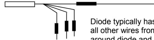
Diode typically has heaviest wire. So twist all other wires from components together around diode and solder and trim so only diode wire extends though. Then crimp male pin to this single wire.
