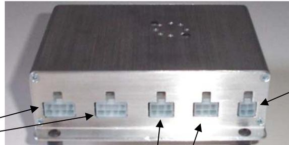
**RPM Inputs** on 6 pin connectors. Right is Engine RPM and other RPM (channels 1 & 4). Left is RPM channels 2 and 3. Both provide access to additional 1 analog channel if the proper breakout cable is used.
