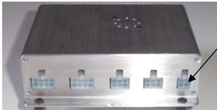
Plug the Switch into the 4 pin connector marked "Switch" on the DataMite III USB logger box as shown to the right.
