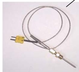
**Thermocouple Channels.** Thermocouples are used to measure temperatures, like exhaust temperatures, fluid temps like oil and water, air temperatures, etc. They can measure from 0 to 2100 deg F.
