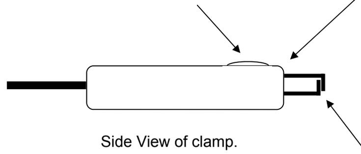
This sensor senses current flowing through the primary (low voltage) wire. The current must be 3 amps or more for it to trigger. If it is not triggering (reading RPM), there may not be enough current for your application.
