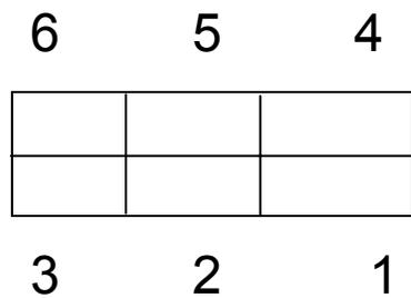
Typical 6 pin connector attached to cable to this type RPM sensor. Pins 1 and 4 are typically connected to this sensor. Pin 6 may be present but is not used for this type sensor.
