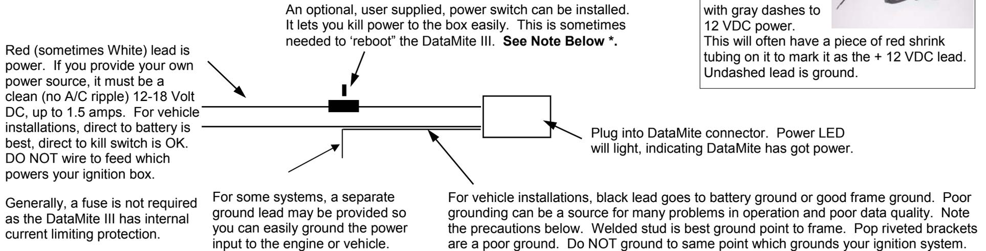
\* Note: For best results, it is best to start and stop recording with the Record Switch (lighted toggle switch). You can start recording by switching on power with the Record Switch in the Record position. HOWEVER, you can NOT stop recording by just switching power OFF, because the box will not be able to write an "end of file" mark on the recorded data file.
