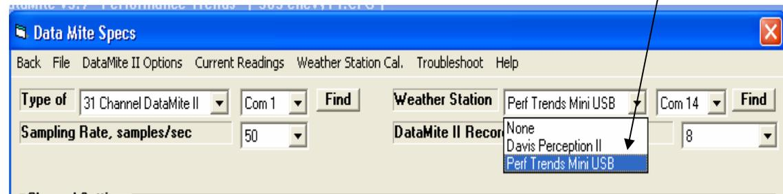
Be sure to set the correct Com Port for this weather station. Click on the Find button to see what the possible ports could be.
