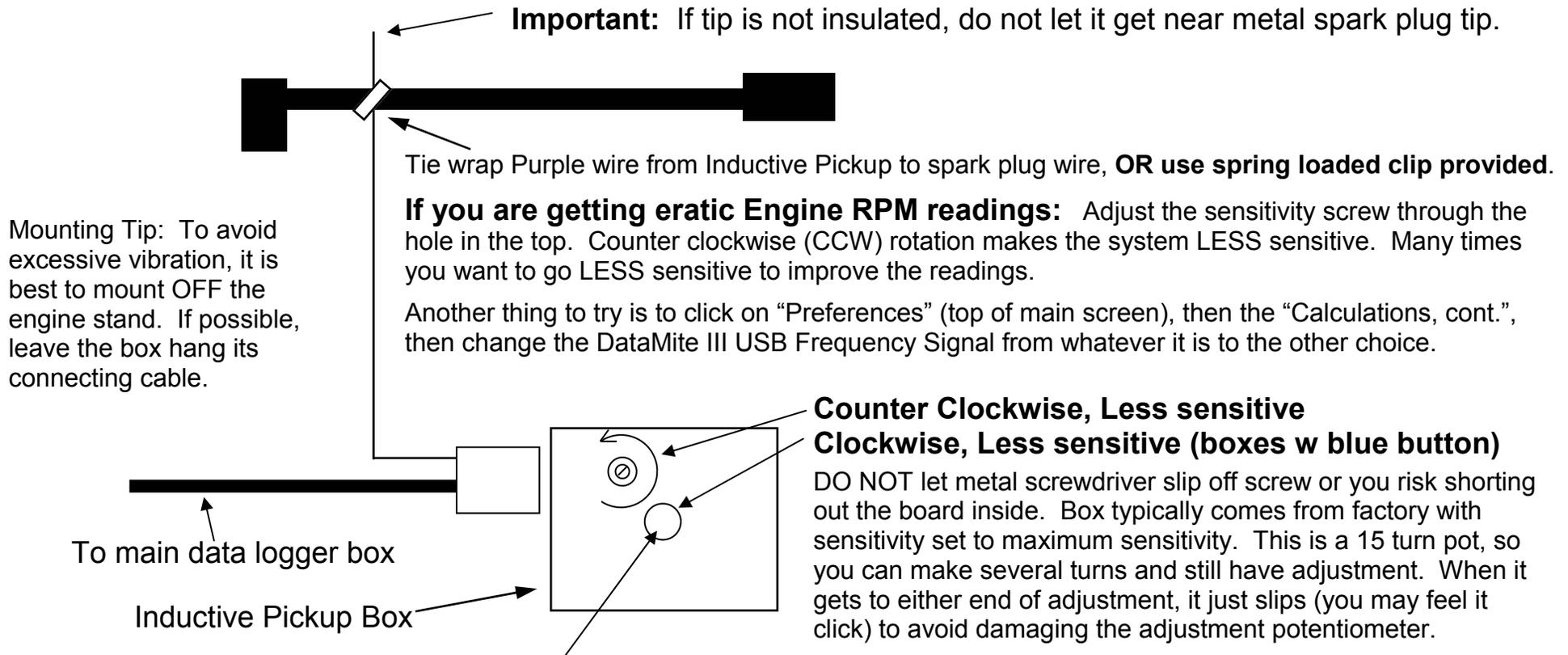
Blue button on newer boxes just indicates the sensitivity screw reverses (CW makes less sensitive).
