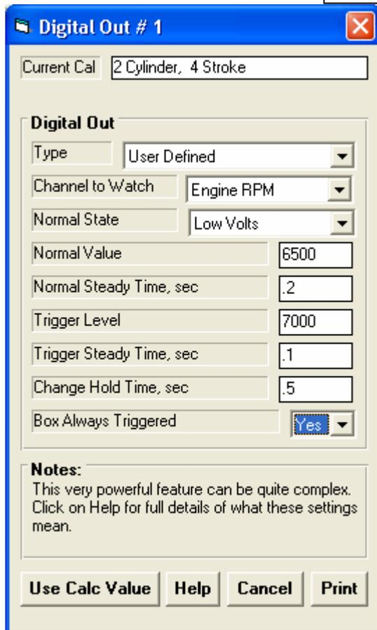
Choose one of the **Type** options and most settings are disabled. The remaining inputs make your choices easier for the typical user. Choose User Defined to enable all settings. (Tip: Choose a predefined Type to fill in most inputs, but then change to User Defined to do minor customizing.)
