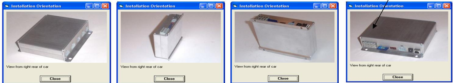
Mount the box as vertically if on edge or level if mounted flat as possible. Mount the box as parallel to the vehicle's centerline as possible.
