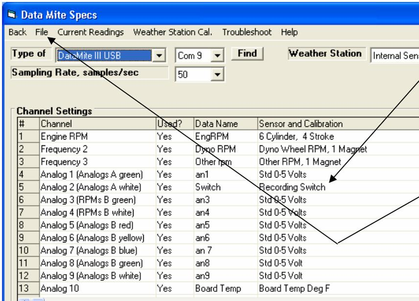
You must assign one of the analog channels as a Recording Switch.
