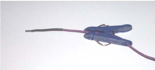
2) Now open clip and insert purple wire through hole in clip about half an inch (12 mm). Then allow clip to close some and pull wire back through hinge and hole in finger pad.
