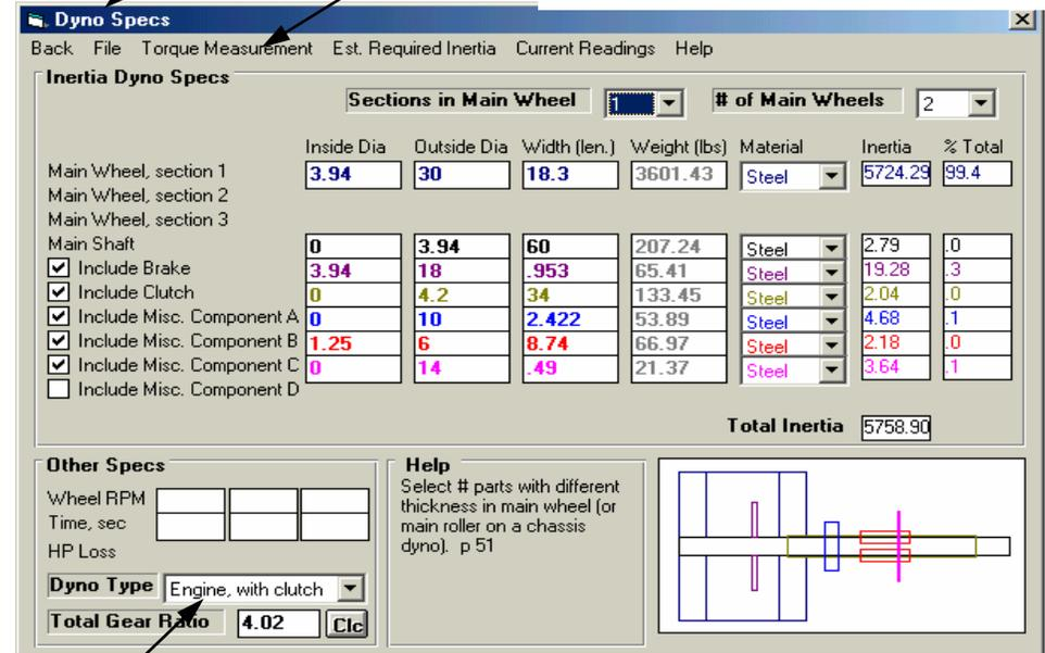
Dyno Type setting determines if you will measure both engine and dyno RPM, or if you need to. We recommend you select:
