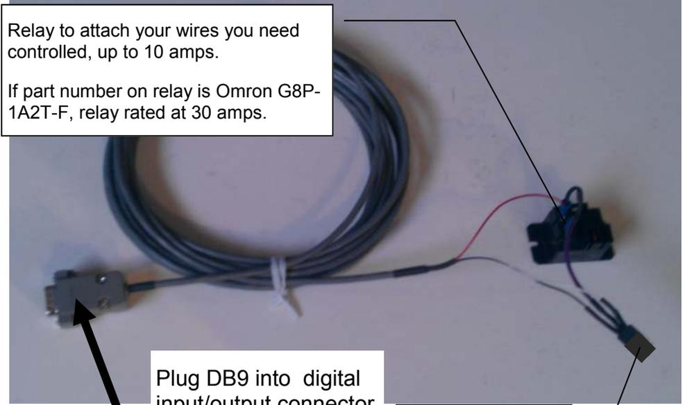
Relay to attach your wires you need controlled, up to 10 amps.
