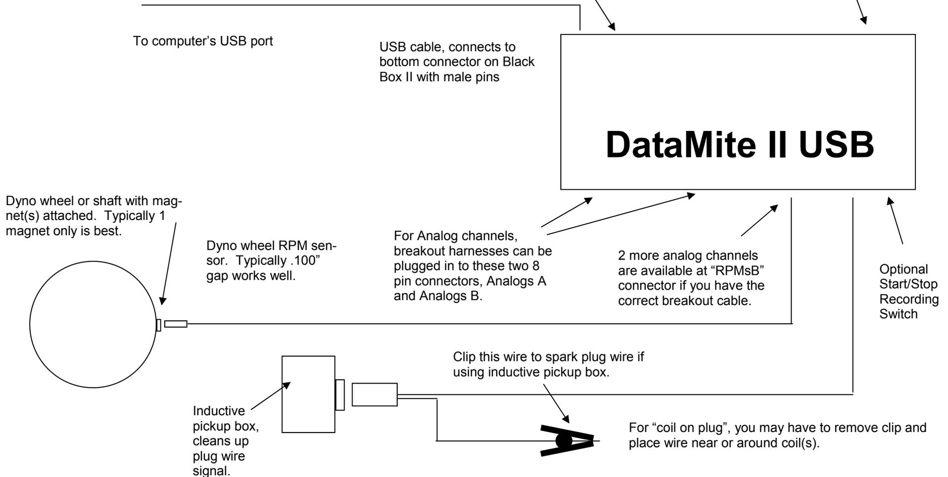
For "coil on plug", you may have to remove clip and place wire near or around coil(s).
