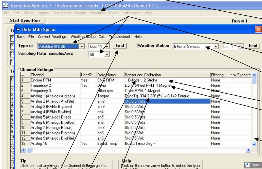
Configure DataMite III Channels by first clicking on DataMite at top of main screen.
