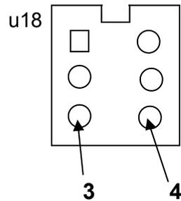
Push capacitor legs through holes 3 and 4 as shown to right, turn board over and solder legs in from below. If left longer, you could short out capacitor on enclosure.
