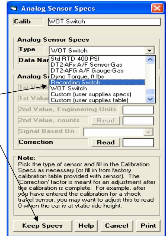
Plug the Switch into one of the analog channels. **DO NOT** plug the switch into the 4 pin connector marked "Switch" on the DataMite III USB logger box. That is for a vehicle switch.
