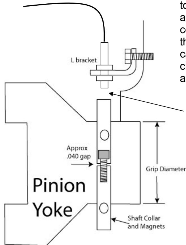
**IMPORTANT:** You must install the sensor bracket on something that moves with the driveshaft yoke. This picture shows you mounting it to the rear axle housing and the rear axle yoke. You **CAN NOT** install the collar on the transmission Yoke and the bracket on the underbody of the car, because the clearance will change with suspension movement and vibration.
