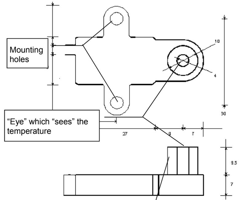
Cylindrical, aluminum heat reference for the IR temperature sensor. When mounted, this should NOT touch any metal components for best accuracy.
