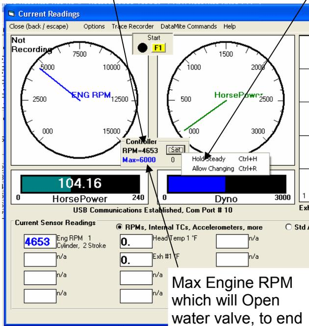
Max Engine RPM which will Open water valve, to end the test. This is set
