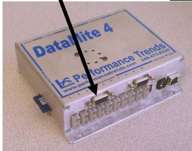
Control wires from DataMite 4 connected to smaller terminals. They can be connected to either terminal, no polarity.
