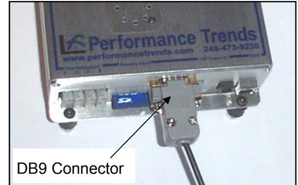
Plug the other end of the cable into the DB9 connector on the DataMite III USB box.
