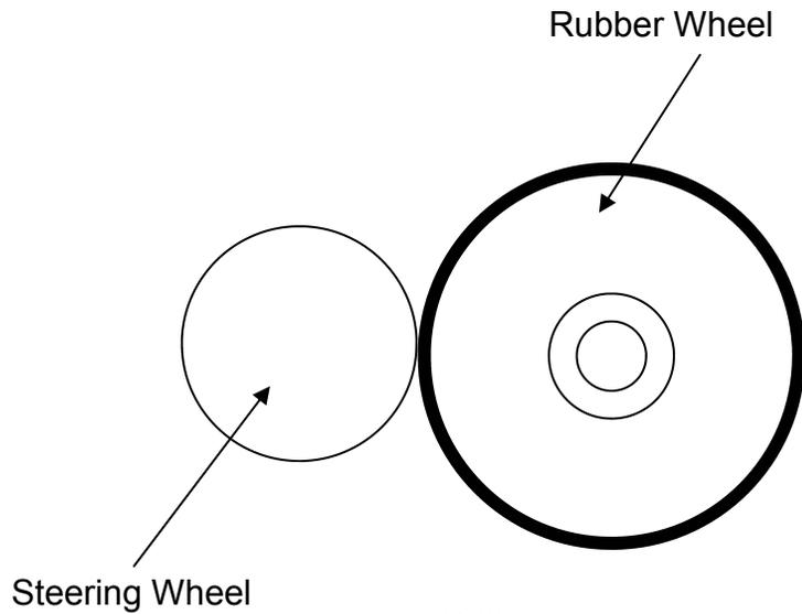
With vehicle wheels pointing straight ahead, install sensor with rubber wheel 1.5 turns from one end of travel. Sensor has 3 turns, so turn to a stop, then turn
