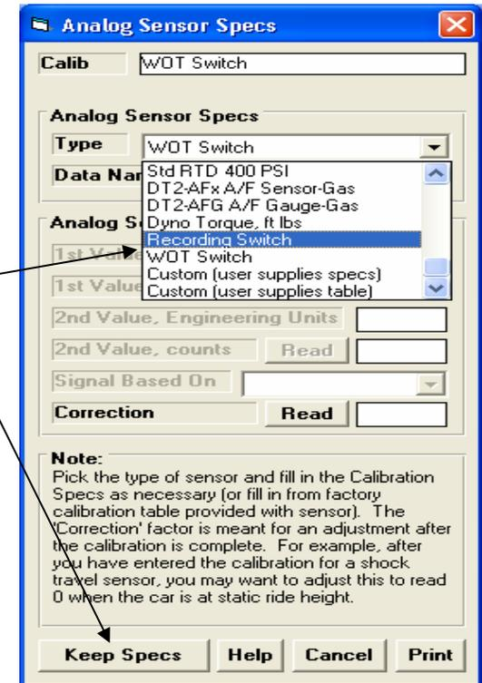
Note that WOT Switch is also an option. When using this calibration, this input does NOT start or stop the recording. You must do that via the F1 and F2 key. This switch just marks exactly when the engine is Full Power (Wide Open Throttle). When this switch is pushed now marks what part of the test will be used for doing power curves.
