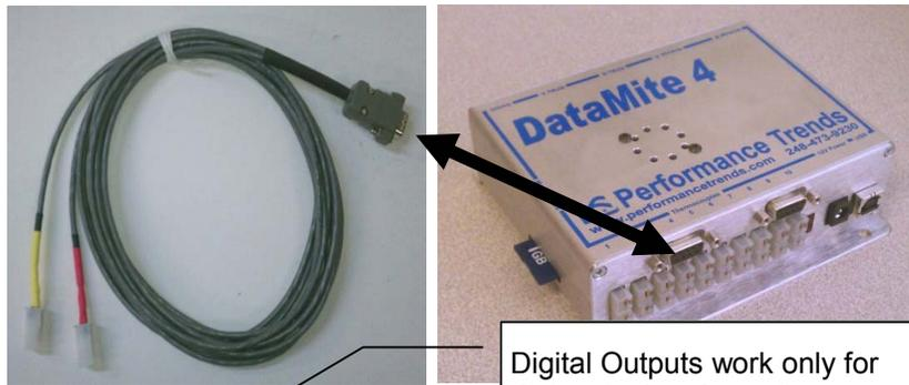
Digital Outputs work only for DataMite 4 w Pro software
