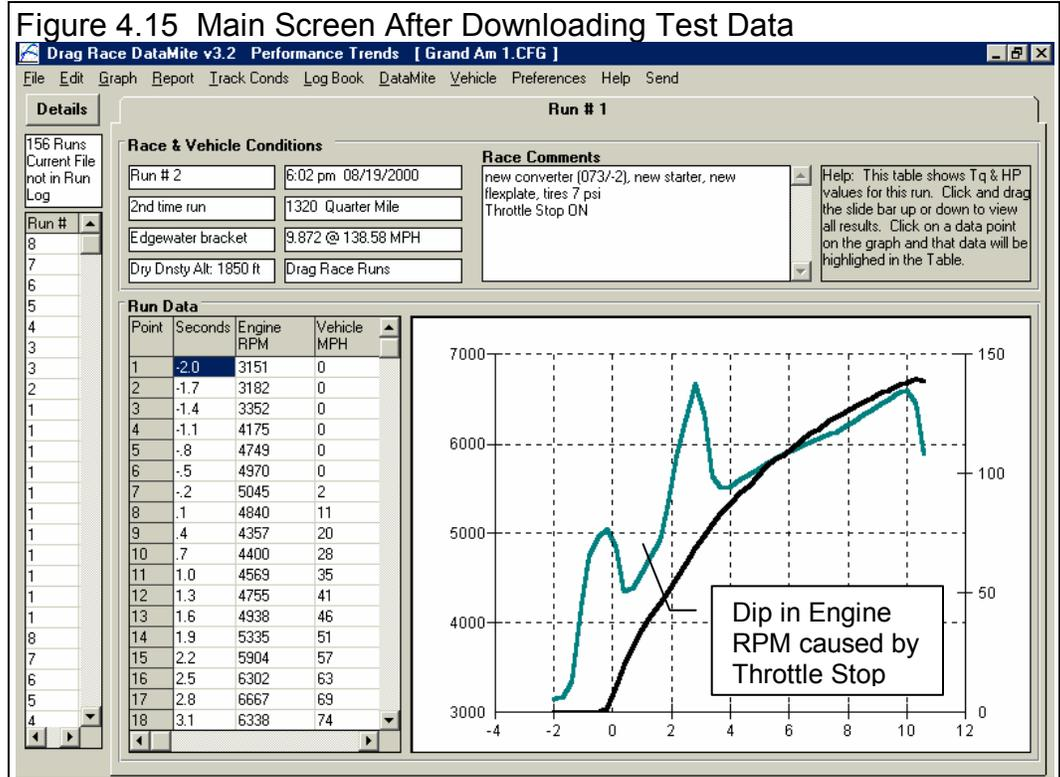
The Grand Am is running a throttle stop, which is why there is such a large dip in Engine RPM right after the launch.
