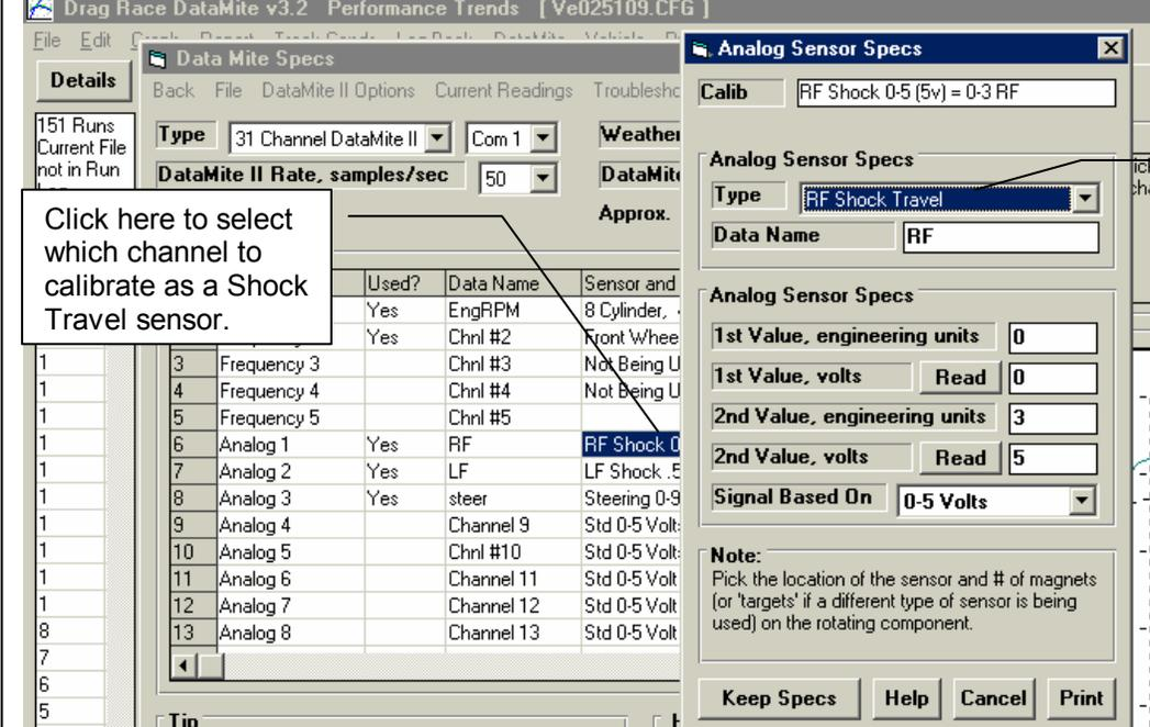
The screenshot shows the 'Analog Sensor Specs' dialog box. A callout box points to the 'Type' dropdown menu, which is set to 'RF Shock Travel'. The text in the callout says: 'Click here to select which channel to calibrate as a Shock Travel sensor.' Another callout box points to the 'Type' dropdown with the text: 'You must select one of the 4 Shock Travel sensor types, or Steering, for that data to be recognized as the appropriate data for the suspension analysis program.'
