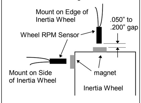
magnets insures more accurate, less "noisy" RPM data.
