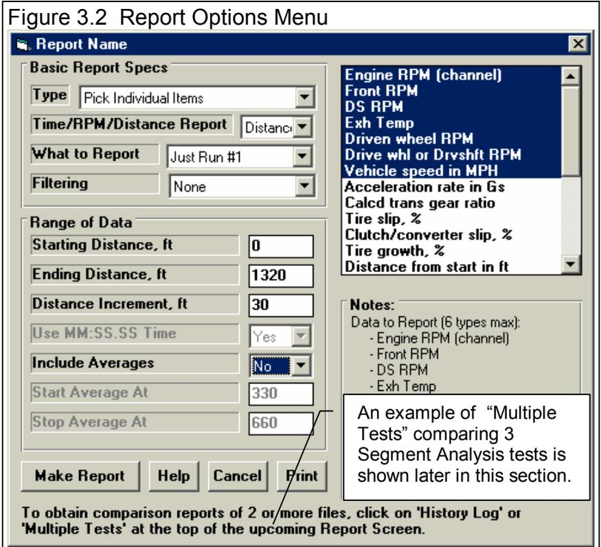
For reports, filtering is not as critical as for graphs. Lets say you specify reporting data at, 250 RPM increments. If your report includes 4500 RPM, then all data within that 250 RPM increment (from 4375 - 4625 RPM) is averaged together to make the number you see reported at 4500. This averaging process is much the same as filtering
