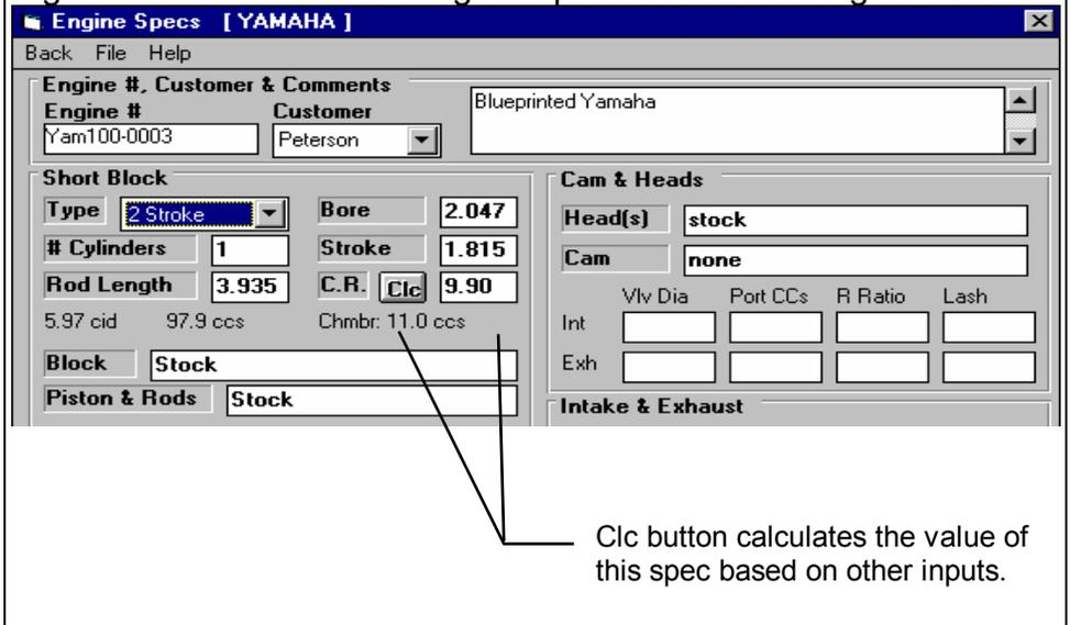
Clc button calculates the value of this spec based on other inputs.
