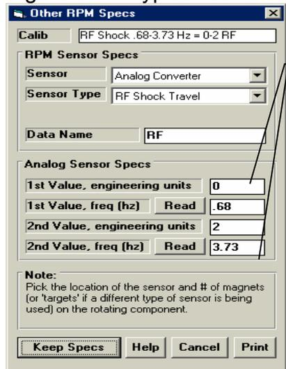
When calibrating, these values are the either the Shock Sensor motion for Susp. Anzr or Wheel motion for the 4 Link Calculator program.
