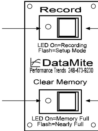
Push Record button to pause recording data (Record LED goes Off). Push Record button again to resume data recording (Record LED comes back On).
