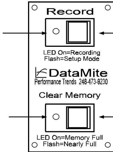
Setup Mode starts with displaying channel #1, engine RPM. Push Record button to Channel #2, and again to display Channel #3, etc.
