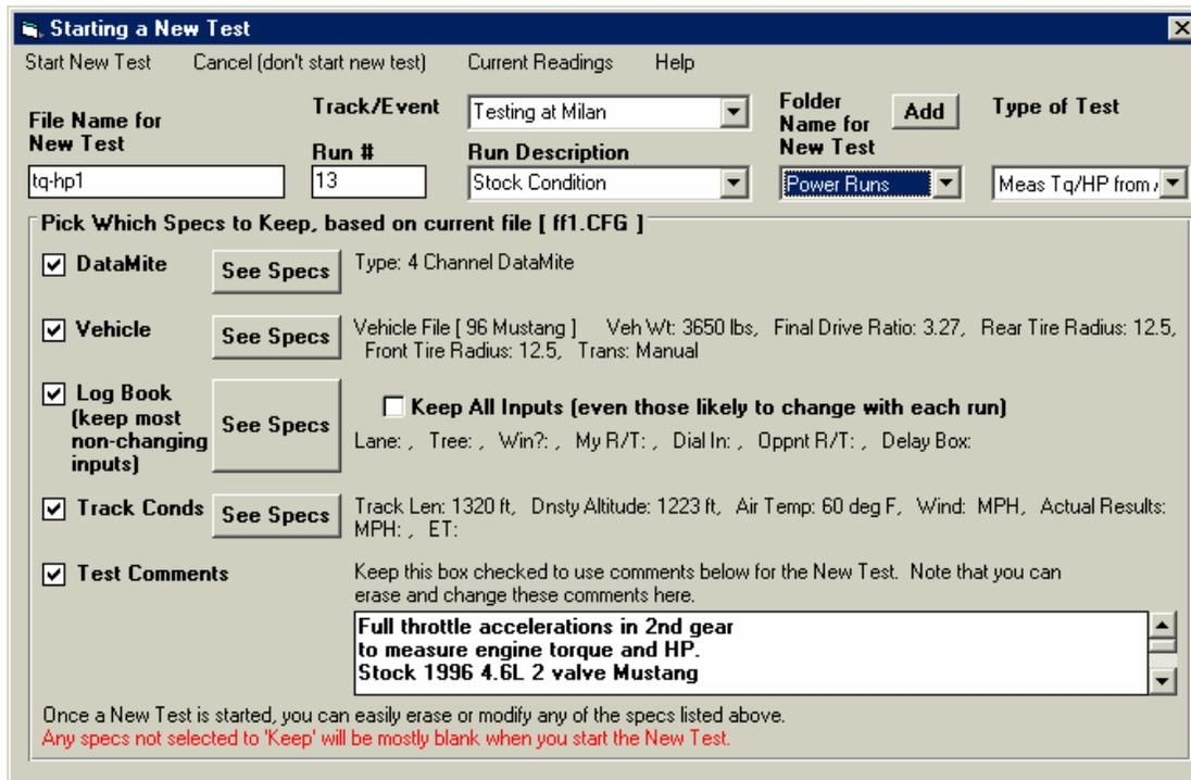
You give the new data file the name TQ-HP1 and save in a new folder name called “Power Runs”. Adding a new Folder is done by clicking on the Add button by the folder name in the New Test screen. You also pick the Type of Run as “Meas Tq/HP from Accel” from Accel“ from the list of possible types. The program says 1 run has been found which is 10 seconds long, which looks correct.
