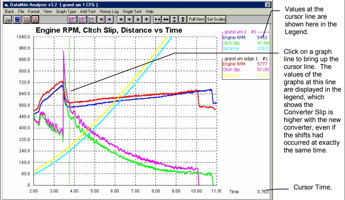
Figure 4.29 Analyze a Section of a Graph with 2 Cursors
