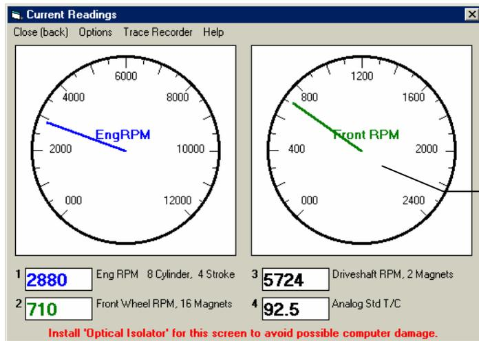
Current Readings screen for 4 channel DataMite
