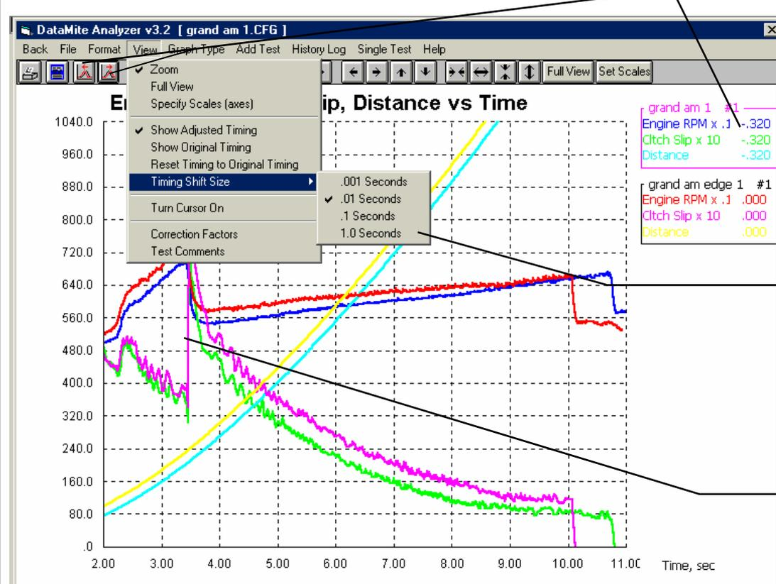
Click on these Time Align buttons to shift one of the tests over another. The amount of shift is shown in the legend. Grand Am 1 had to be shifted back .32 seconds for good alignment with the "Edge" test
