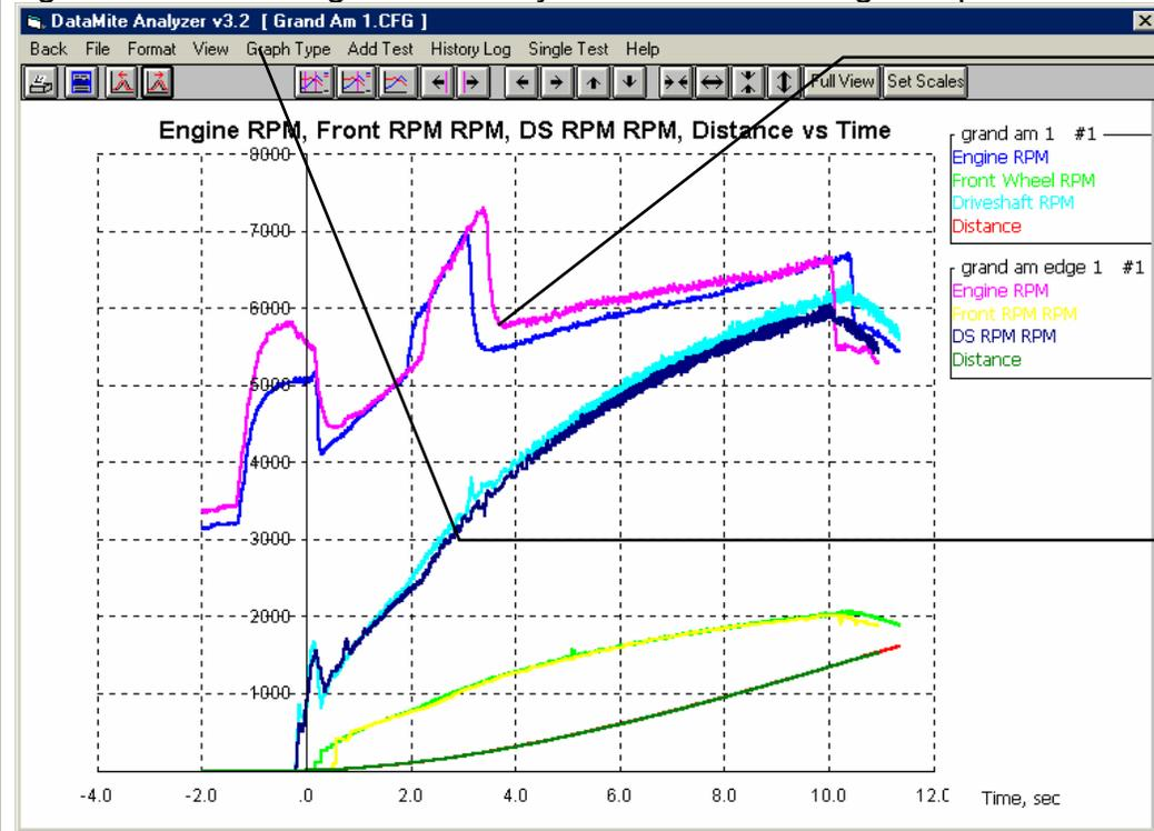
Both runs look quite “clean” (no noise spikes) and quite similar. The biggest difference is with Engine RPM. “Grand Am 1” with the new converter seems to have lower Engine RPM throughout most of the run, possibly being a “tighter” converter.
