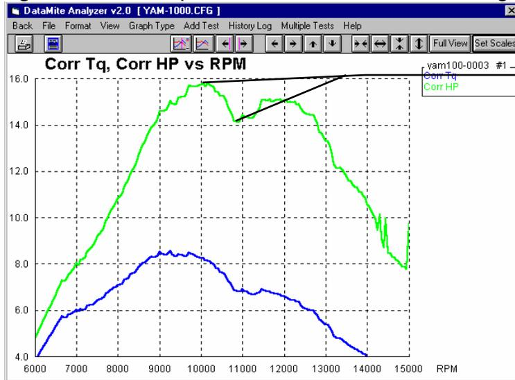
Note that the peak is the highest and the valley is the deepest when filtering is the least, in this case None. These torque and HP graphs look fairly smooth, even with Filtering = None, so even None would be an acceptable for these torque and HP graphs.
