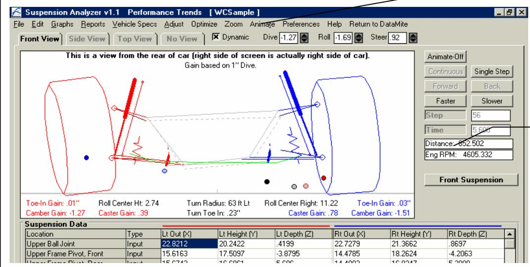
You can manually start displaying DataMite data by clicking on Animate and selecting DataMite data file as Data Source.
