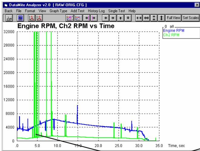
Data After Editing Out 32 Noise Spikes (many Noise Spikes remain, too many for accurate torque and HP calculations)
