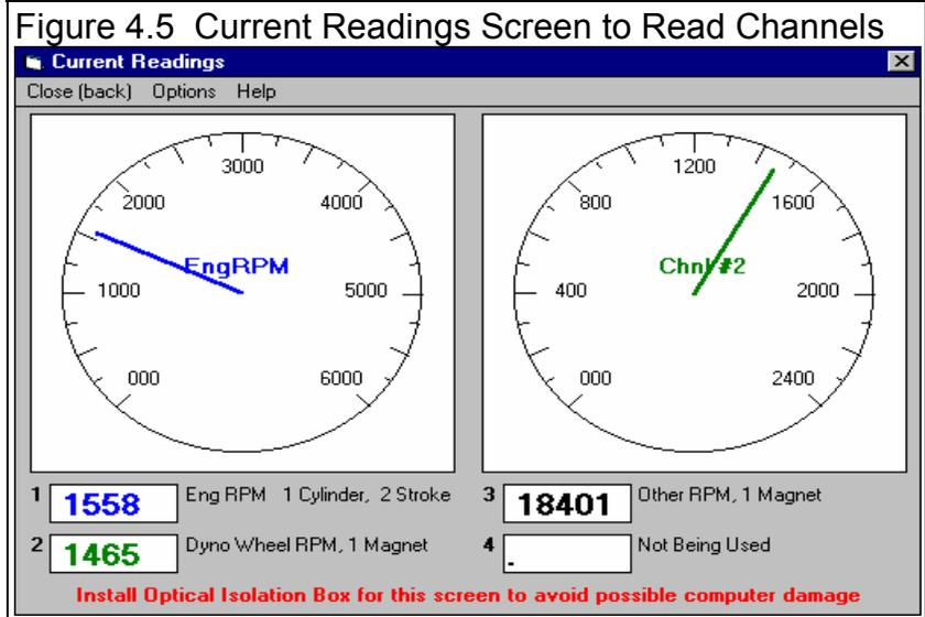
**Note:** It is recommended you use screen only if you have protected your computer's serial port with Performance Trends' optical isolation system. Although unlikely, it is possible for "stray" high voltage ignitions signals to pass back through the DataMite and destroy your computer's serial port.
