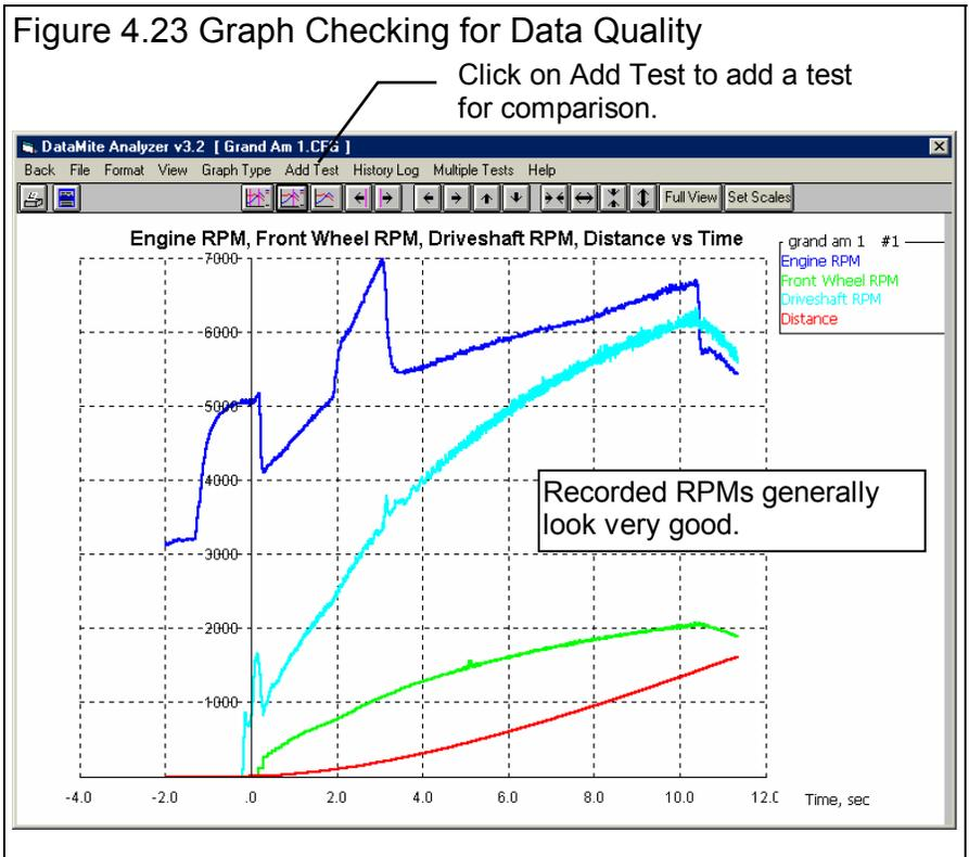
Now add the test you want to compare this test to by clicking on Add Test in the Graph Screen. See Figure 4.23. You will obtain a screen similar to Figure 4.21 on the previous page. Select the Grand Am Edge 1 test, which had been run at a different track (Edgewater) with the old converter. You should now obtain a screen similar to that shown in Figure 4.24. The Grand Am Edge 1 has nothing that looks like a noise spike, so its data quality looks very good also.
