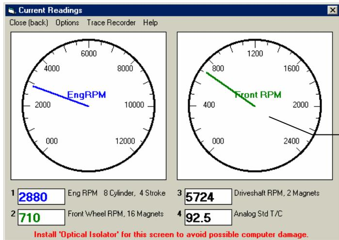
Current Readings screen for 4 channel DataMite
