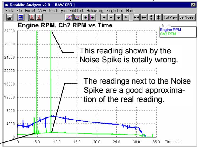
If many Noise Spikes occur close together, the program can not accurately determine if a spike is "noise" or real data, and leaves it in.
