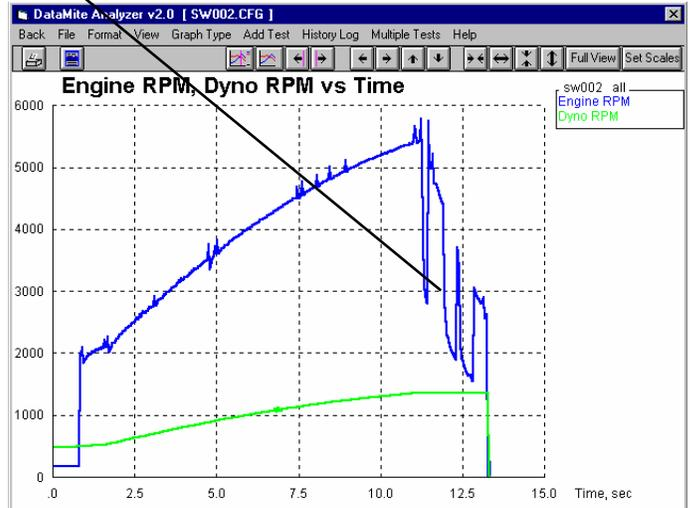
If the inductive pickup signal is too strong (you wrap the spark plug wire too many times), you may not be able to record Engine RPM at high RPM. Engine RPM may drop in half or all the way to 0 RPM.
