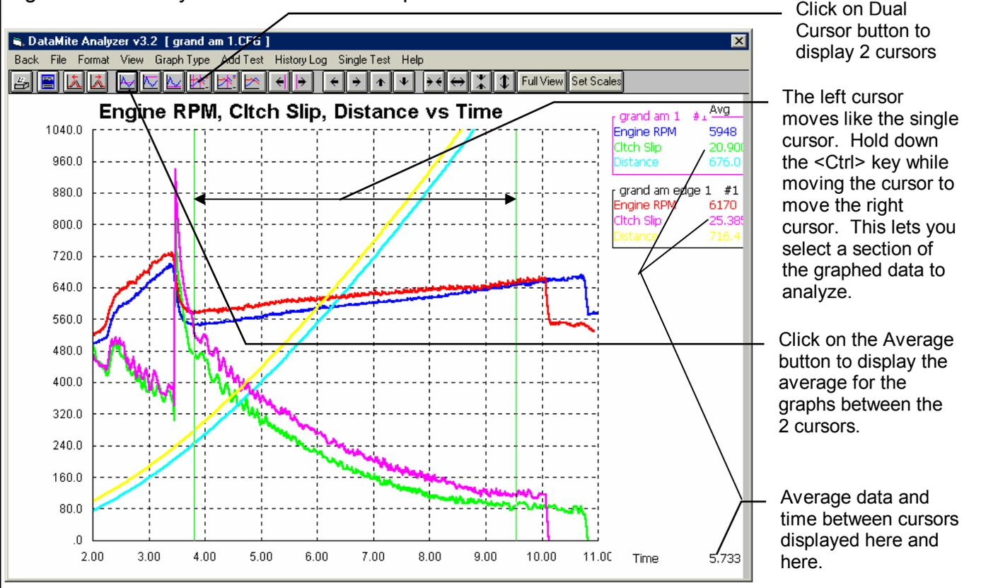
Figures 4.25 through 4.29 show how you can use graph features like Time Aligning, Zooming, Cursor and the Dual Cursors to check various performance characteristics.
