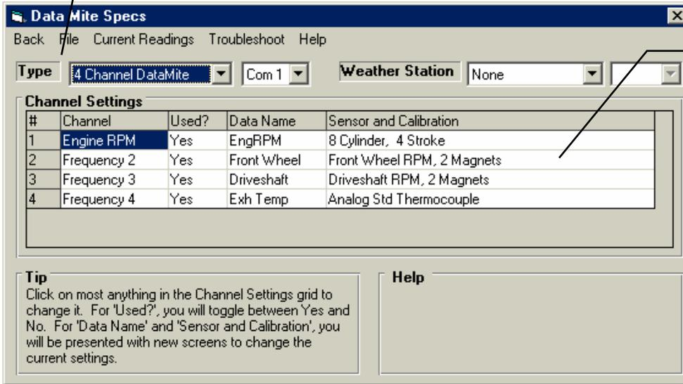
Click here to bring up the Sensor and Calibration screen for defining each channel, as shown in Figures 2.21 and 2.22.
