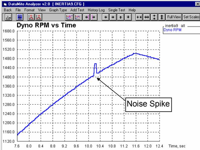
Typical "noisy" or "jumpy" data shows all data points being quite different than the surrounding data points. In this case the "noise" is due to magnets on the shaft not being exactly evenly spaced.
