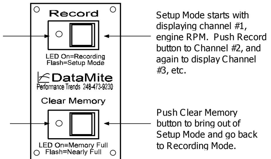
Figure 2.4 DataMite Recording Mode
