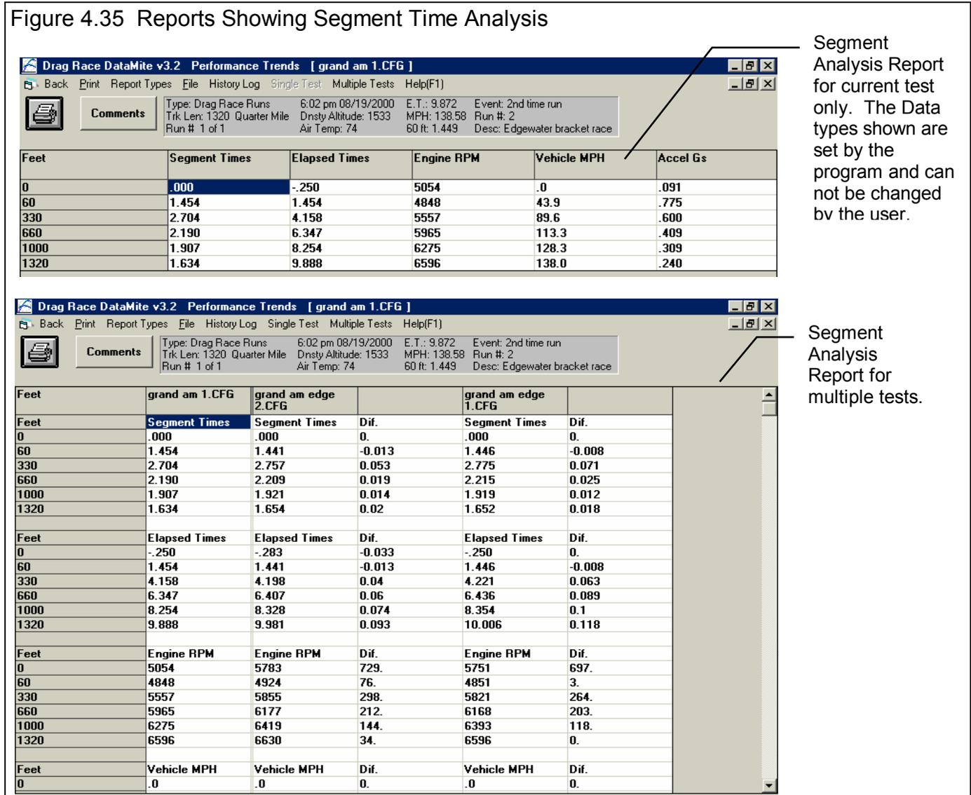
Segment Analysis Report for current test only. The Data types shown are set by the program and can not be changed by the user.
