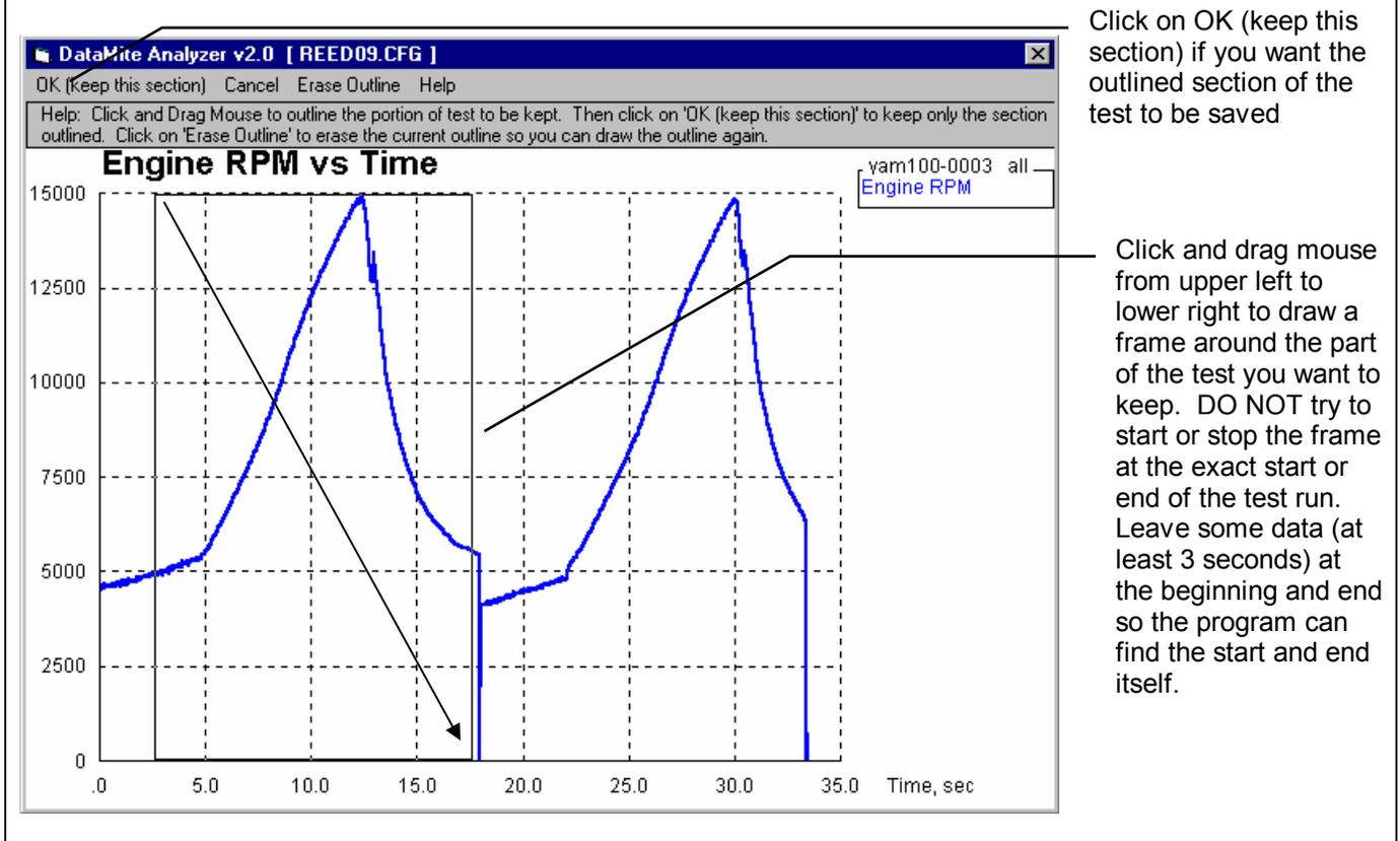
If you click on Edit, then Delete Beginning or End of File, you will be presented with a graph screen showing Engine RPM for the this entire test. Click and drag the mouse to draw a square frame around the portion of the test you *want to keep*. The rest of the test will be deleted. When you are satisfied with the section you've drawn, click on OK (keep this section) to be presented with the options shown in Figure 2.47.
