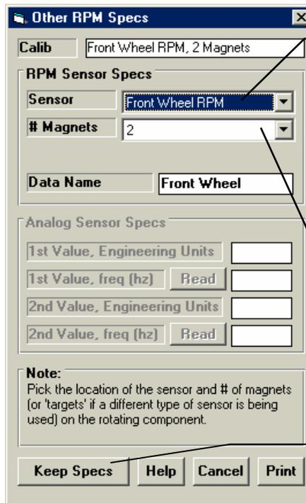
Pick Front Wheel for channel 2 and Driveshaft RPM for channel 3. You would open this menu twice, once for each channel you want to change.
