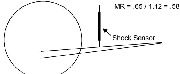
Side view of rear ladder bar with shock sensor
