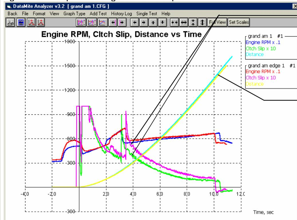
Rather large difference in Converter Slip, with the new converter bring “tighter”.
