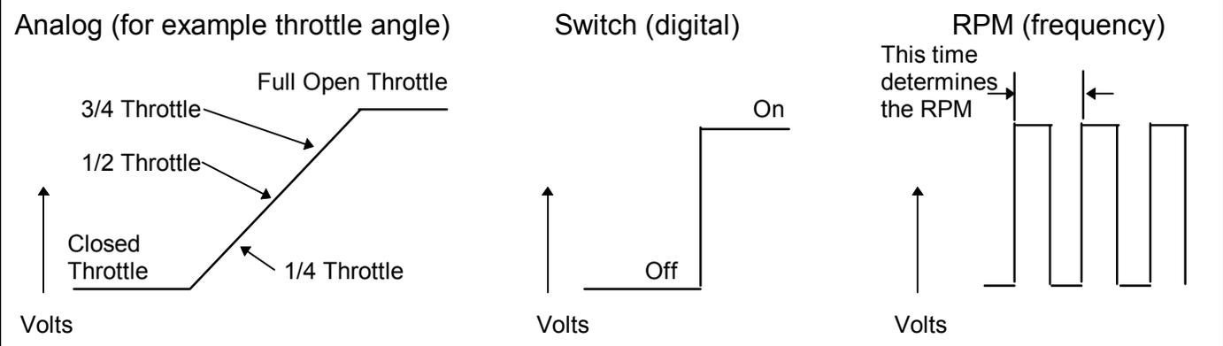
Switch Sensors and RPM Sensors do not require much calibration. Tell the program if either high or low voltage is opened or closed, or On or Off and the switch channel is calibrated. Just tell the program how many pulses you get on 1 revolution of a shaft, and the RPM channels are calibrated. These 2 types of channels are not usually in error just some. It is usually very obvious if there is a calibration error (like specifying the wrong number of magnets on the dyno inertia wheel).
