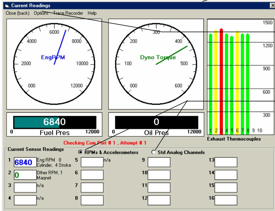
Current Readings screen for 30 channel DataMite II
