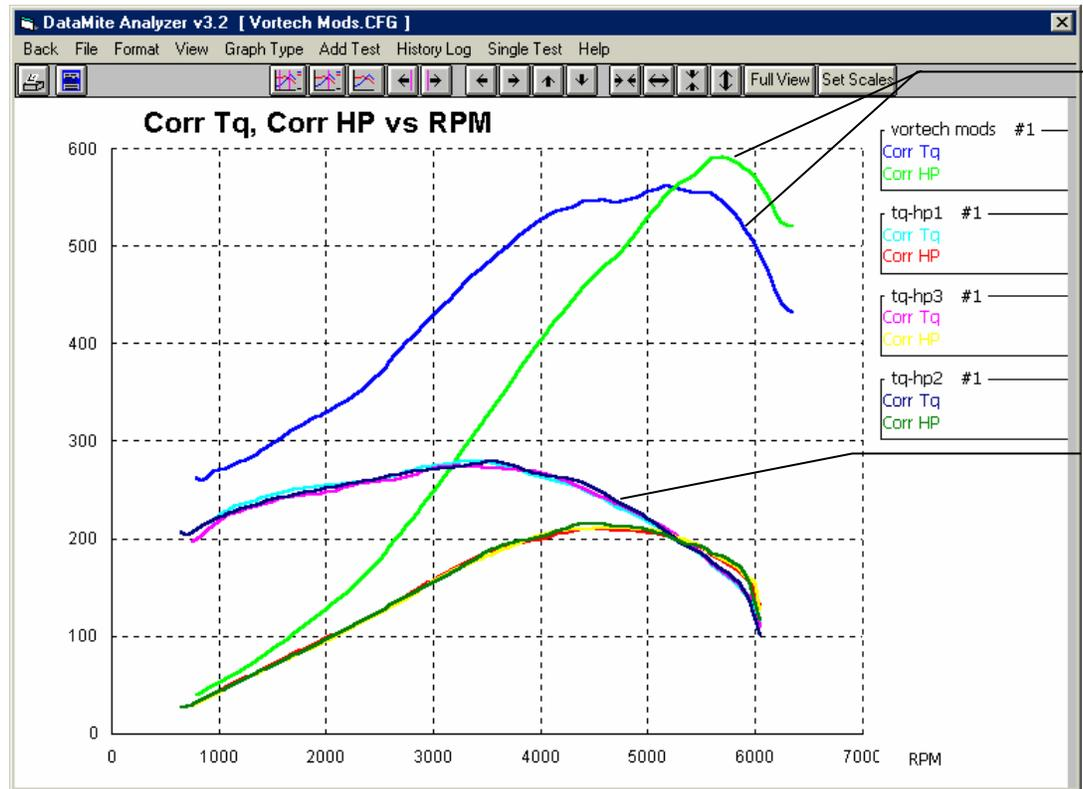
Torque and HP curves from doing accels after adding a Vortech supercharger and other mods, showing huge increase.
