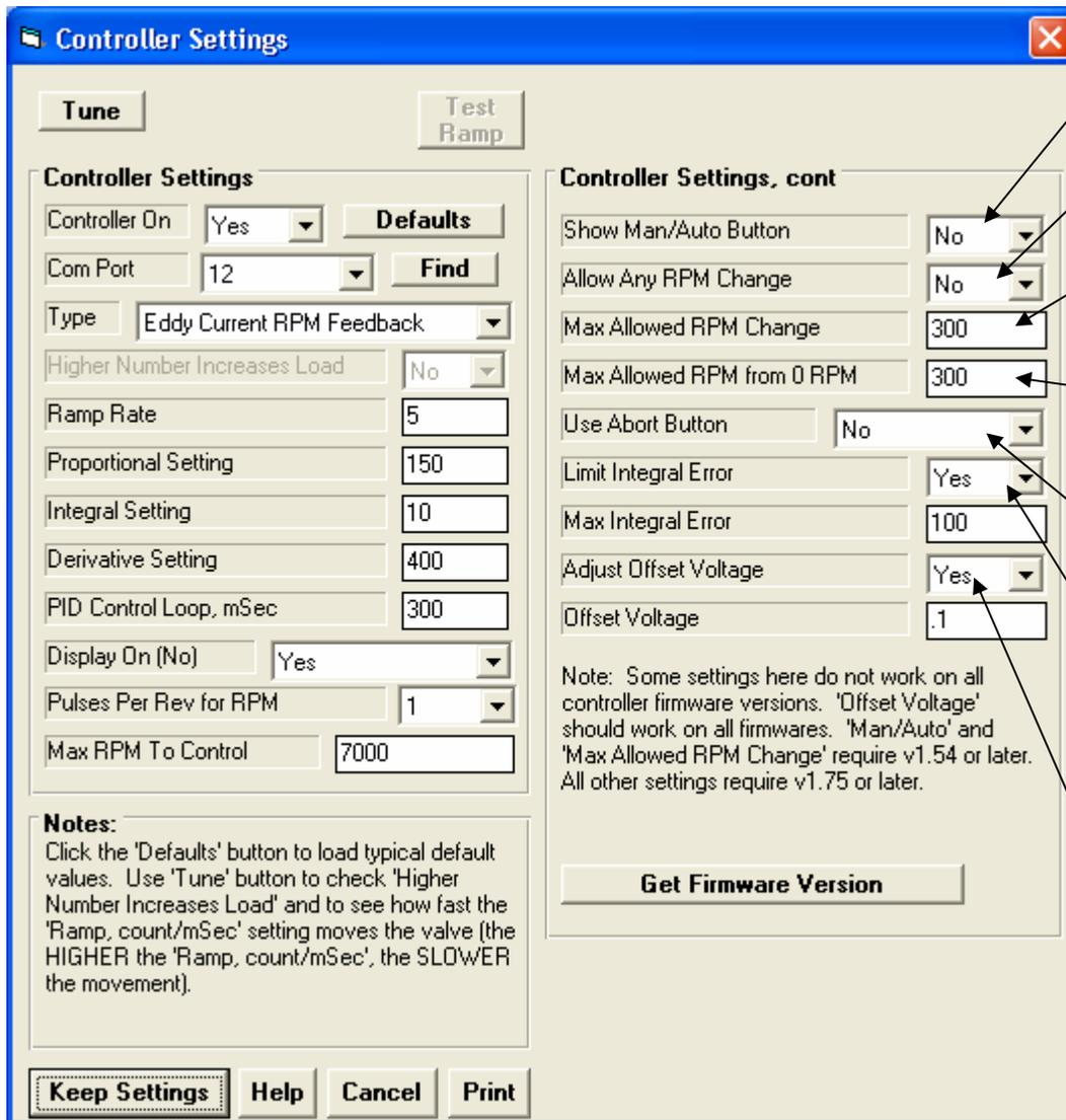
Choose Yes and the screen shows either Auto (control to RPM) or Man (vary dyno absorption power directly) depending on pressing a button on the controller.
