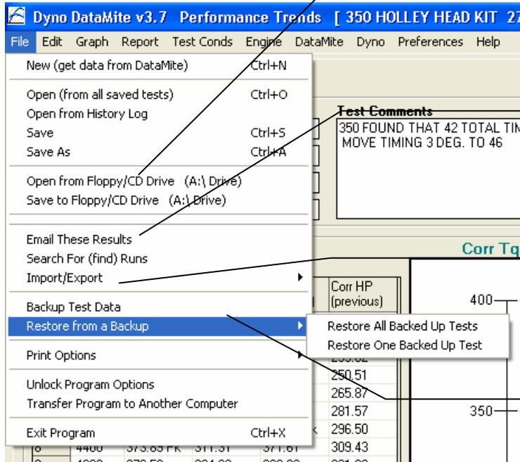
Saving To and Opening From an External Drive (floppy, CD or memory stick) makes it easier to transfer individual tests from one computer to another.
