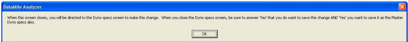
In this case, the Master Dyno specs needed to be updated. When you close out the Test Conditions screen, the program automatically opens up the Dyno Specs screen, and automatically enters the needed change (Dyno Type = "Chs Dyno, no eng RPM" in lower left). When you close this screen, it asks if you want to save the changes as the Master. . Typically you will answer Yes.
