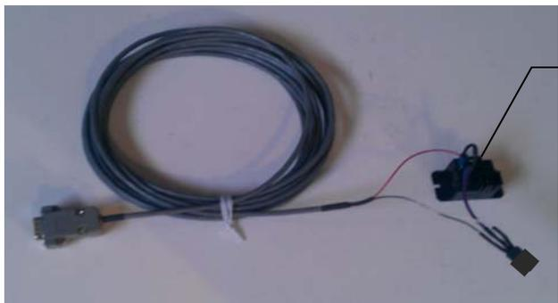
Hardware shown here is a 20 amp relay with a relay driver. This could be used for turning a motor, fan, or ignition power On or Off.
