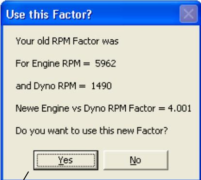
If you click it, the program grabs an Engine RPM reading (if available) and Dyno RPM reading. The program asks if the Engine RPM reading should be used. For example, if low engine RPM is accurate, but high RPM is not (spikes or dropouts), you could do this calibration at lower, accurate Engine RPM and use the measured Engine RPM and answer Yes.
