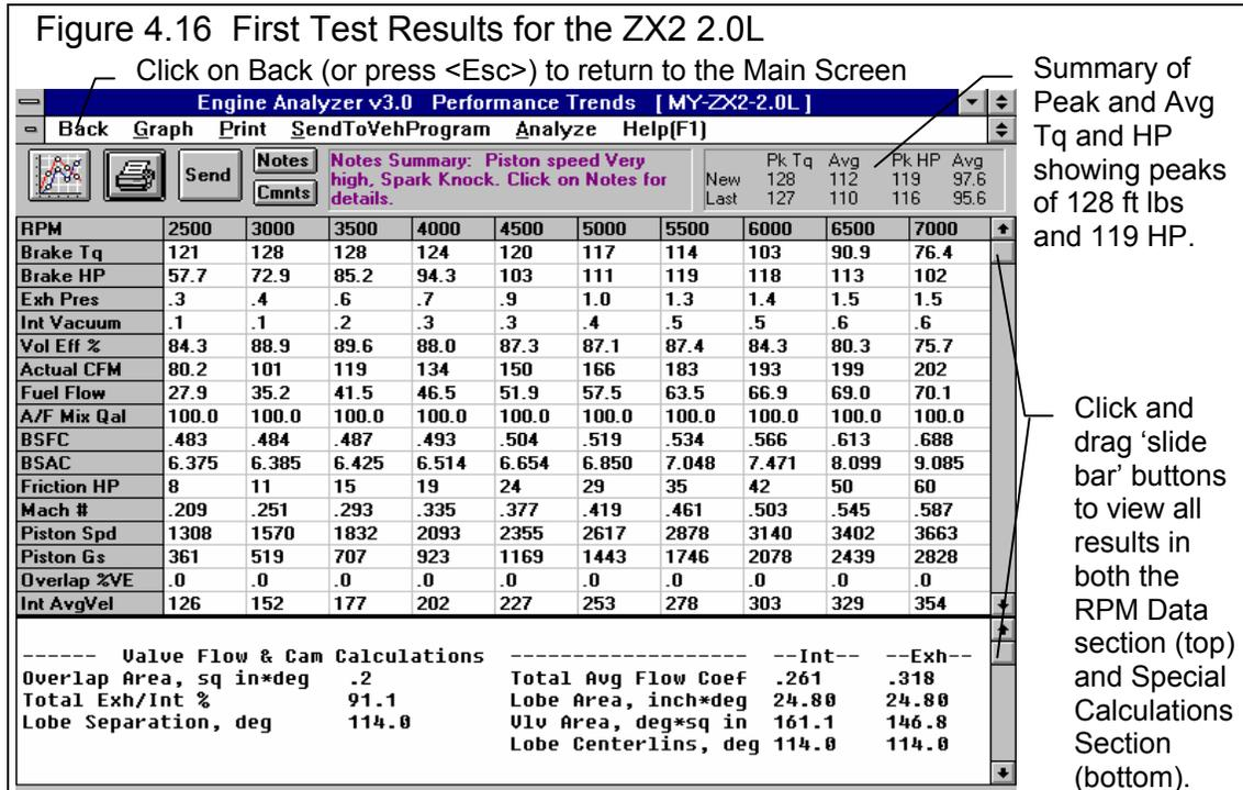
The program first checks your inputs to be sure there are no obvious problems, things like valve sizes being too big to fit into the bore size, etc. If no problems are noticed, calculations will proceed and you will obtain the results screen shown in Figure 4.16. You may initially be given some Engine Analyzer Tips as shown in Figure 4.4, page 153. Read them and then click on OK.
