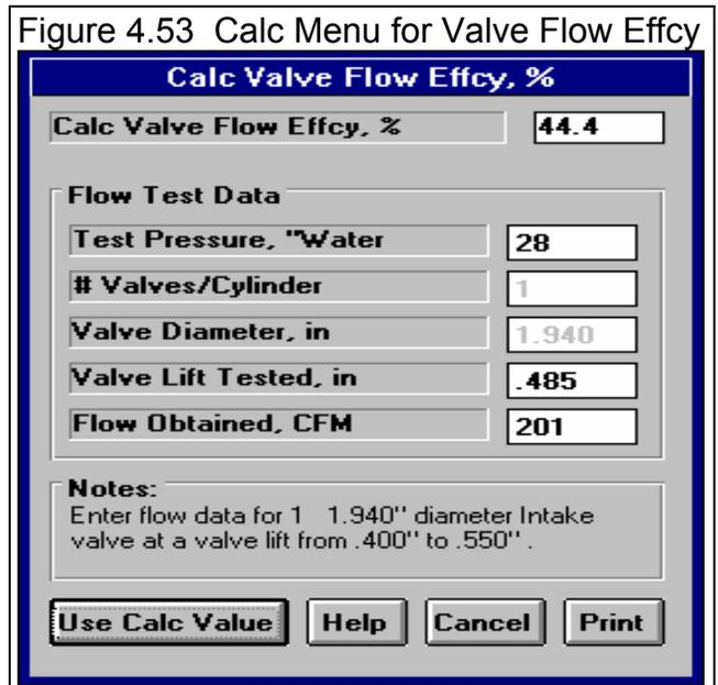
The changes to the Head(s) specs should now be 1.54" Avg Port Diameter, 152 Port ccs and 44.4% Valve Flow Effcy, all for the Intake Port. Click on OK to close the Head(s) menu.
