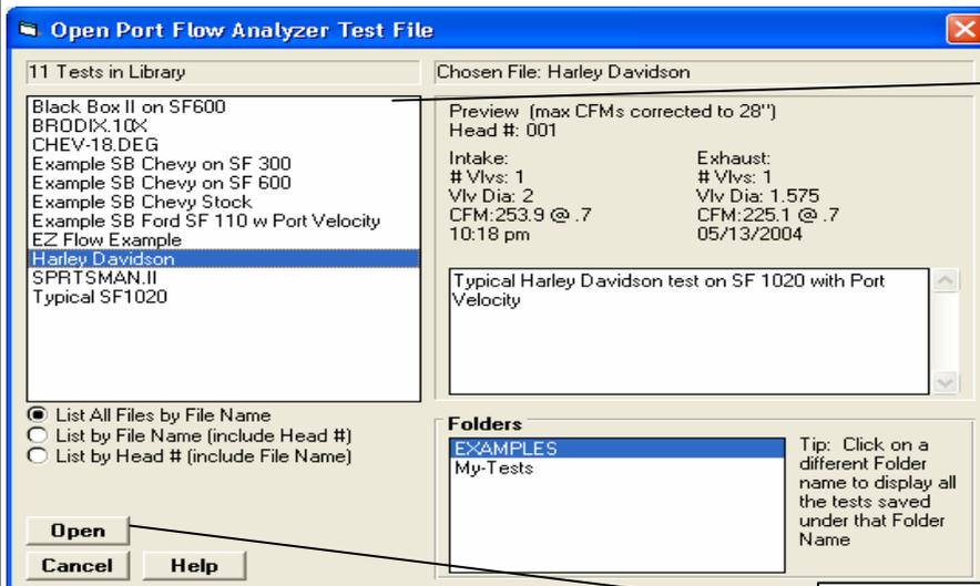
You get this screen by clicking on the "Load Files from Port Flow Analyzer" button shown in Fig 11. This screen is very similar to the File Open screen in your Port Flow Analyzer. Use it to choose the file you want to load.
