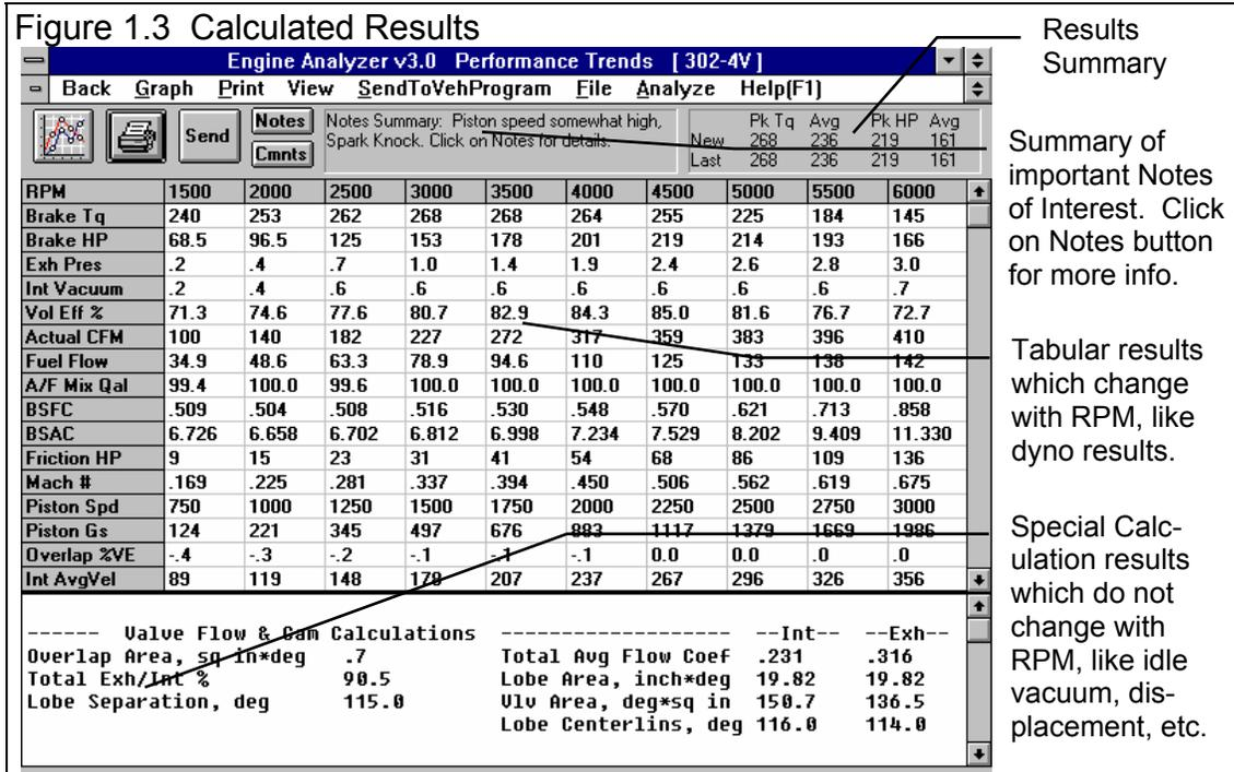
The final results will appear in a table as in Figure 1.3. The rows are for various types of readings (Brk Tq, Brake HP, etc) which occurred at the RPMs you requested in the Running Conditions menu.
