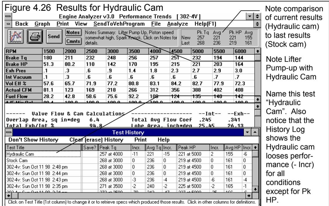
Note comparison of current results (Hydraulic cam) to last results (Stock cam)
