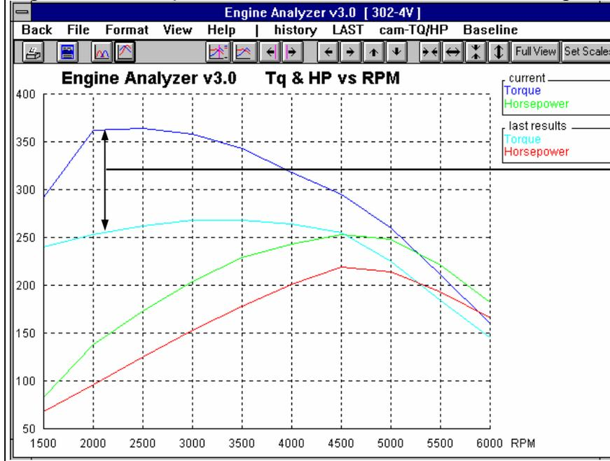
Note large gain in low RPM torque, and that performance with the small turbo increased at all RPMs.
