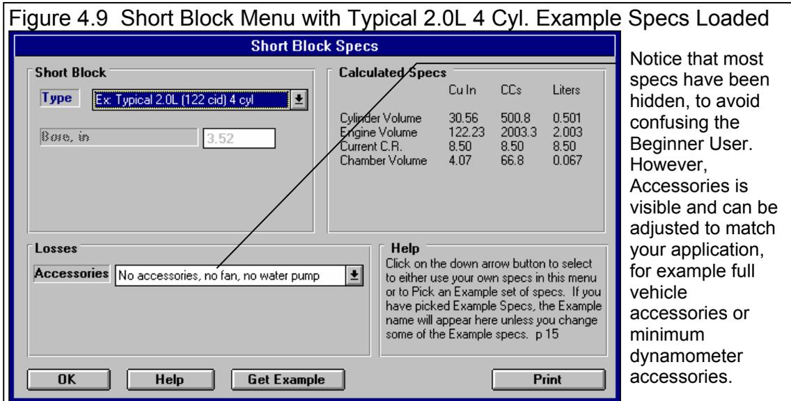
Notice that most specs have been hidden, to avoid confusing the Beginner User. However, Accessories is visible and can be adjusted to match your application, for example full vehicle accessories or minimum dynamometer accessories.
