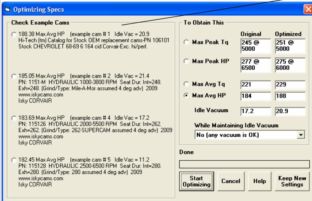
The program will show the 4 best cams which meet your criteria. Pick one of these 4 using the round option button, then click on the "Keep New Settings" button to load in this Example Cam.
