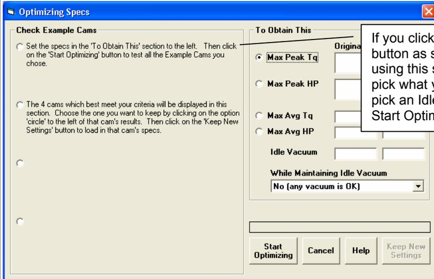
If you click on the "Optimize Using These Cams" button as shown in Figure A 16, instructions for using this screen are displayed here. Basically you pick what you want to optimize (Max Peak Tq, etc), pick an Idle Vacuum level, and then click on the Start Optimizing button.
