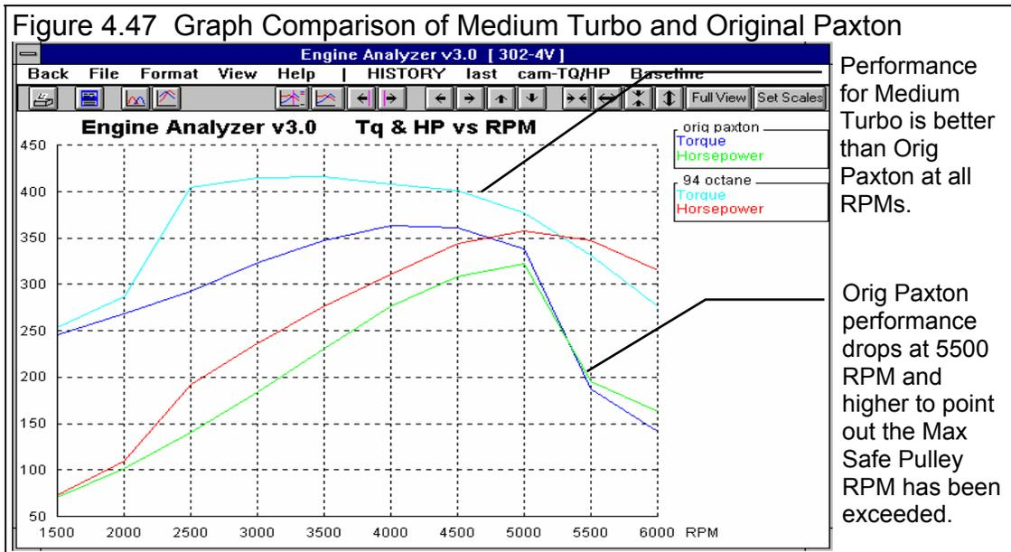
The results from both Figure 4.46 and 4.47 show performance for the Original Paxton being down significantly compared to the Medium Turbo. However, compared to stock, Peak HP has increased over 100 HP. Another interesting thing in the results is that Friction HP has increased significantly. For example at 5000 RPM it went from 86 HP for the turbo to 110 HP with the supercharger. This extra Friction HP is primarily for the power required to run the supercharger.
