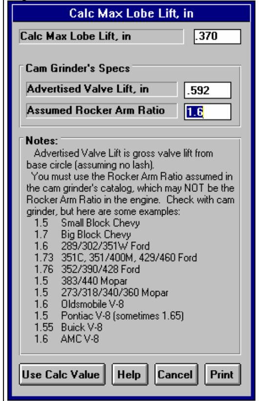
Figure 4.30 Cam/Valve Train Menu for Solid Roller Cam
