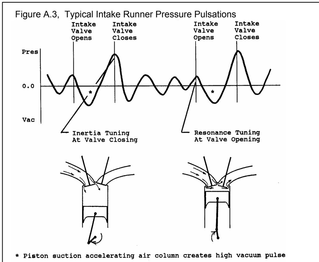
A good analogy of inertia tuning is the "water hammer" effect in old plumbing when you quickly close a running faucet. (New plumbing has "trapped air shock absorbers" to reduce this effect.) Decelerating the column of water in the pipes by closing the valve causes a sharp pressure rise that literally "rattle the pipes". This is the same situation as when the intake valve closes.
