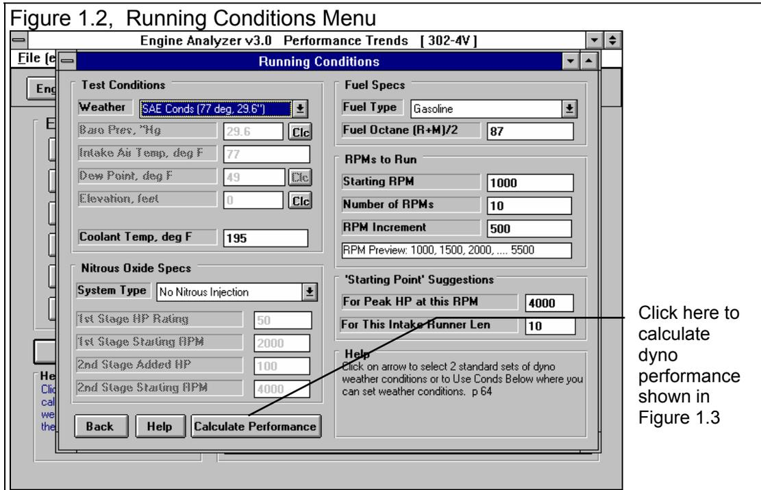
For now, leave all the Running Conditions as they are and click on the Calculate Performance button. This will start the program calculating performance for the specifications of the 302-4V stored in the Engine Library with the Running Conditions currently displayed. A progress bar graph shows how the calculations are progressing. The calculations may require several seconds on slower computers.
