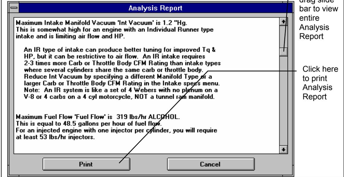
Due to the high RPM, relatively long intake runners, and high overlap camshaft, intake resonance tuning (In ResTunPrs) may be important for this engine. One can see that when In ResTunPrs is high and positive, Overlap %VE is high, Vol Eff % is high and torque and HP are high. Where In ResTunPrs is a high negative number (vacuum pulse during overlap), Overlap %VE, Vol Eff %, torque and HP are low.
