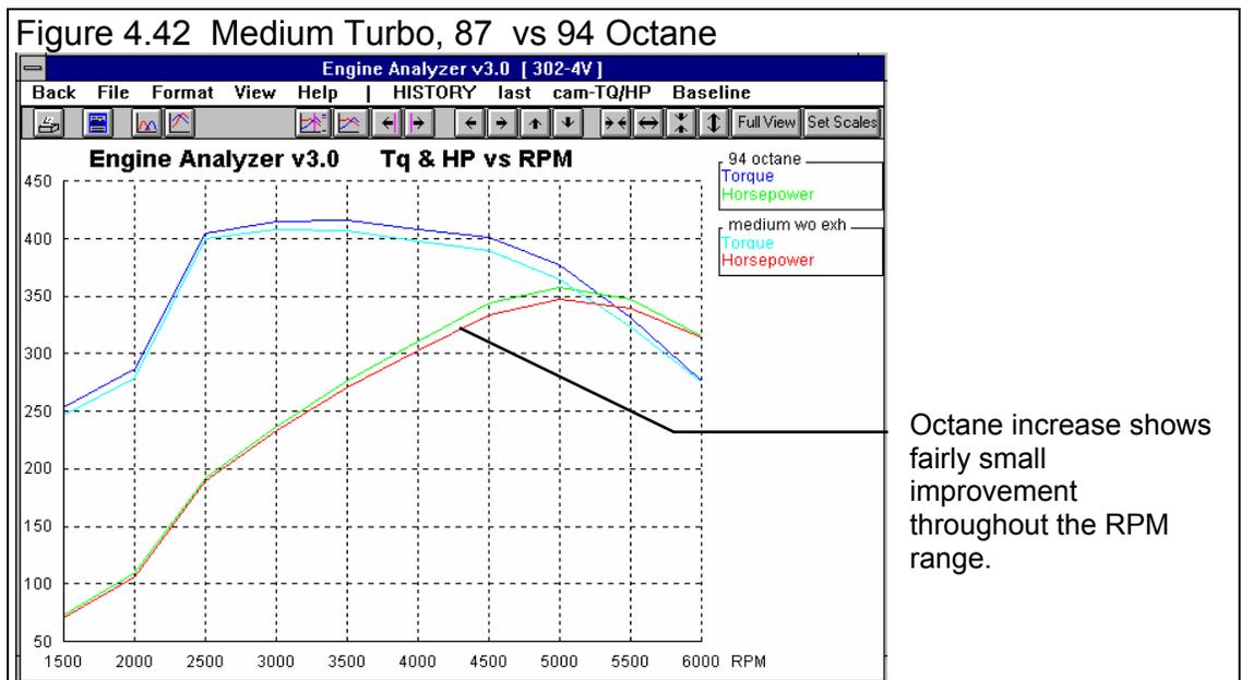
Now that you know that a "Medium" turbo could perform well, you may want to get actual specs from various turbo suppliers and do more precise simulations. You could also load in Example turbos provided in the program by Performance Trends. To see what Example turbos are available, click on Turbocharger Type and select the Pick an Example option, or click on the Get Example button at the bottom of the menu.
