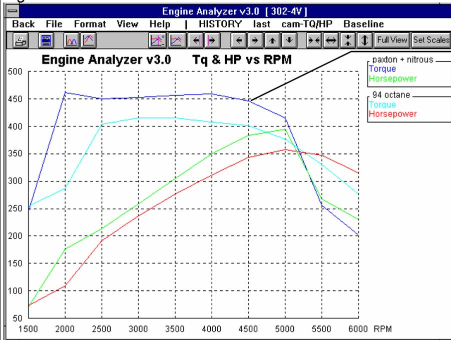
Paxton with 75 HP Nitrous Oxide kit outperforms the Medium Turbo at all RPMs until the Max Safe Pulley RPM limit is exceeded at 5500 RPM.
