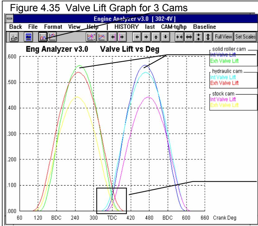
Click here or on Format or on cam-TqHP to produce Valve Lift graph shown here
