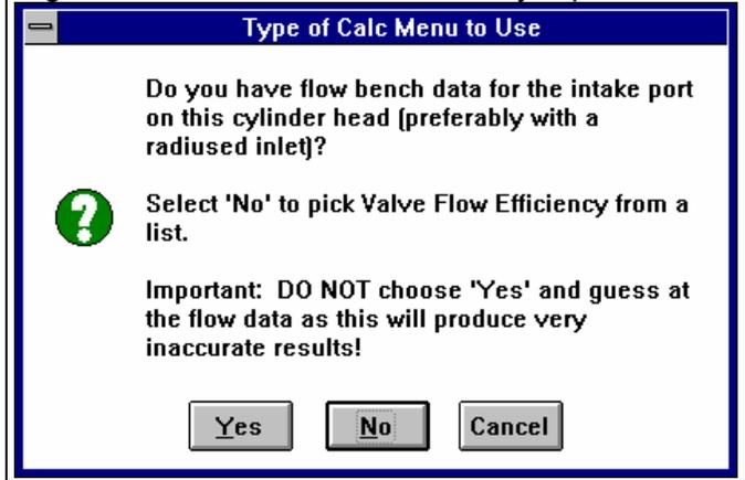
Figure 2.30 Calc Menu to Estimate Flow Efficiency
