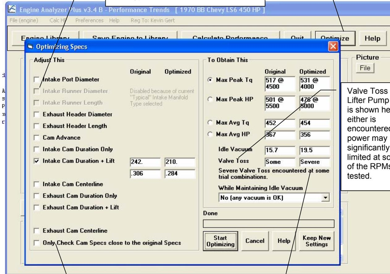
Valve Toss or Lifter Pump Up is shown here. If either is encountered, power may be significantly limited at some of the RPMs tested.
