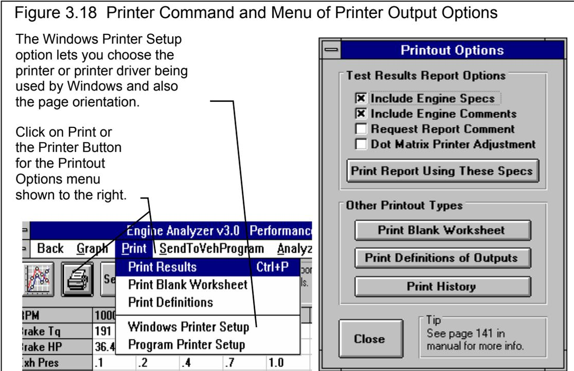
Select this options if you want all the current Engine specs, Transmission specs, etc printed with the results. This will add 1 page to the printed report.
