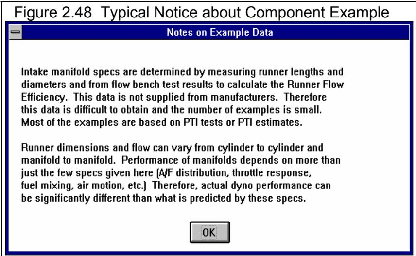
You have the option of changing the Example specs. For example, lets say you have blocked the crossover to your Torquer II and eliminated all coolant flow which could heat the intake. You can click on Intake Heat and select No Heat from the choices. The program will warn you that by changing this spec, the name of the example will no longer be for a Torquer II, but will be changed to the general "Use Specs Below".
