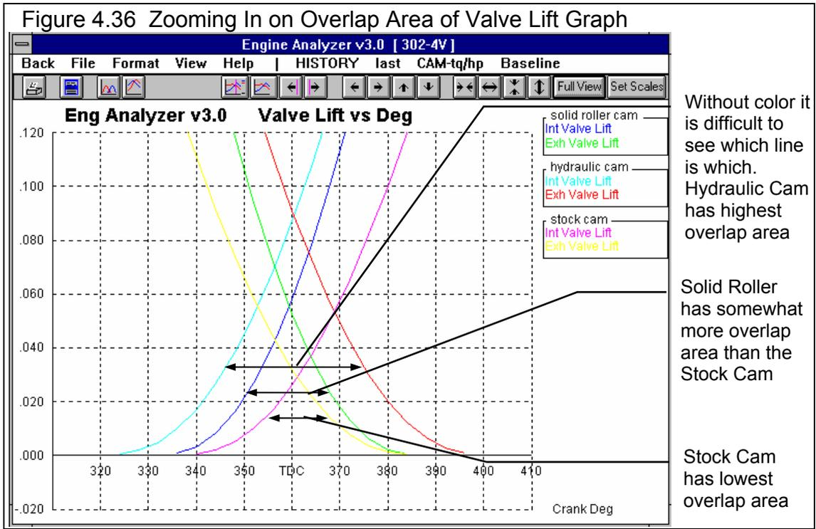
Without color it is difficult to see which line is which. Hydraulic Cam has highest overlap area
