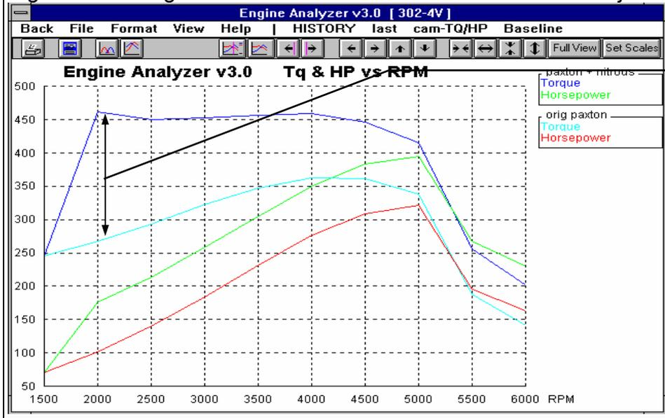
Note the large torque increase at low RPM with the nitrous oxide injection kit.
