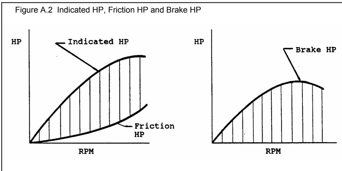
The HP lost to friction can also be expressed as an efficiency:
