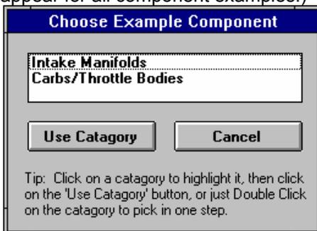
There are 2 general ways to pick an example component. You can either select the Pick An Example from the Type combo box or click on the Get Example button at the bottom of the menu. You may be first presented with a list of general categories of component examples, like shown in Figure 2.45. (This screen would not appear for picking Short Block, Heads or Cams because there are no other component examples available at these menus.)
