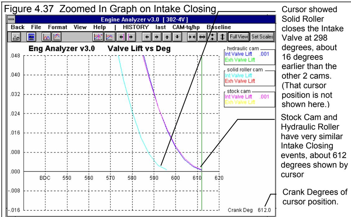
Figure 4.37 shows a zoomed in graph on the Intake Closing ramp of the 3 cams. Using the cursor function you can see the Hydraulic Cam and Stock Cam close at about 612 degrees or 72 degrees after Bottom Dead Center (after BDC on the graph). The Solid Roller Cam closes at 596 degrees, or 56 degrees after BDC.
