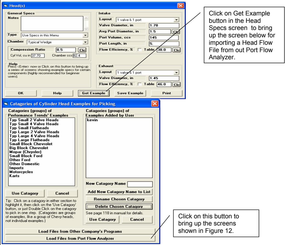
Figure 12 Importing Head Files from Performance Trends' Port Flow Analyzer
