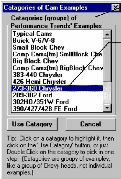
Click on Type in the General Cam Specs, then pick the Pick an Example Cam option to be presented with this menu, a list of categories of cams.
