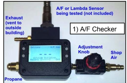
**A/F Checker** lets you check you're A/F measurement system from end to end for accuracy. You provide shop air and propane from a BBQ tank, it tells you the A/F of the mixture and you see if you're A/F says the same thing. Fig 1.
