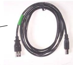
**USB connection** to initially config box (typically not needed) or to check real time readings for setting up sensors or troubleshooting.
