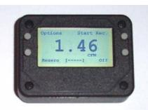
If you have selected to all the Recording Mode, you can press the Start Recording button to start recording blowby. Once recording has started, this label changes to "Stop Recording". Then you press this same button to stop recording. Click on the Options button, then Recording, then Playback to display the recorded blowby data.
