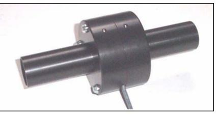
Hook up the blowby sensor to your valve cover following the instructions with your sensor. Hook up the electrical lead to one of Performance Trends' DataMite data loggers. Pick the built in Blowby Sensor calibration for your range of sensor and you're ready to test measure the CFM of blowby from your engine at all engine RPMs.
