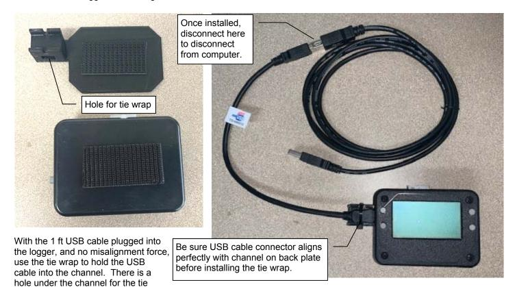
Once this is installed, use the cable connector for plugging and unplugging the logger. Leave the 1 ft USB cable plugged into the logger at all times.
