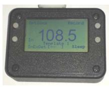
Start turning over the engine with the starter and press the Record button to start recording data. The screen will show "Recording Data". Once enough data has been recorded, the screen will show "Calculating". When finished, the screen will show the Intake Centerline, like shown here. Other options are then available as described in this document.
