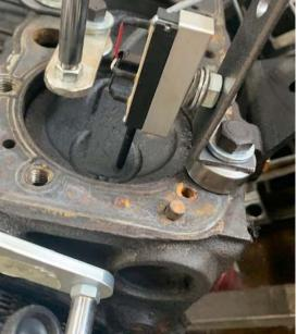
With these adjustments made above, rotate the rotary sensor backward to the start of its rotation and place it on the component turning with the crank. Press the Record button on the QCC logger and start turning the engine over. Try not to go real fast when the piston is near TDC, pressing on the TDC sensor.
