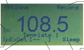
Template Name, shown here as the default "Template 1". Templates are combinations of Rocker Arm Ratios and Lash settings to calculate what the cam lobe specs are if you measure what the valve retainer is doing.
