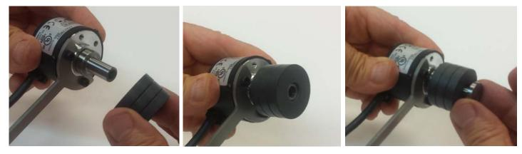
Slide 3 magnets on shaft. Three magnets are used to provide more holding force.
