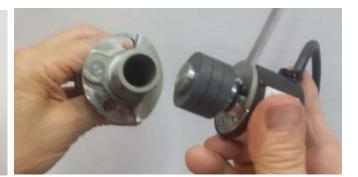
Attach the magnetic hub and insert into the end of your cam. The magnets will hold it in place.
