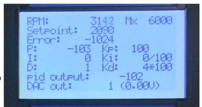
Typically the actual RPM will be slightly higher than Setpoint RPM. This allows the controller to put out a DAC out volts telling the water valve to apply more load. Typically this is with a voltage less than 2.35, like the 1.68 volts shown here.
