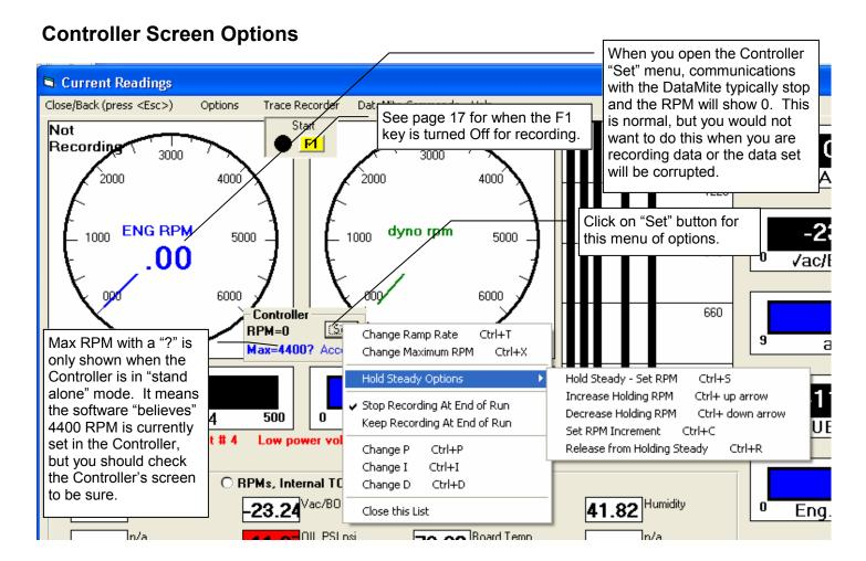
For many options, these are the same as offered in the Controller Setup screen. They just offer a faster, more convenient way of making changes. The "0 Ramp Rate", "Hold" options and "Stop Recording" and "Keep Recording" are new and only available at this screen.
