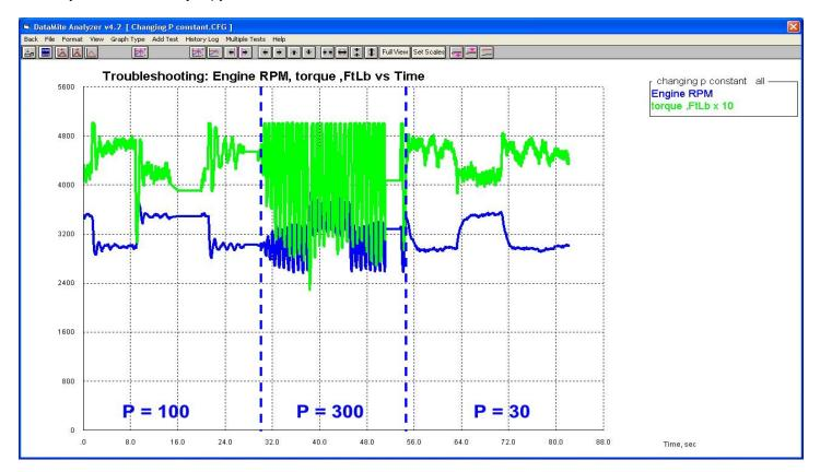
With a P of 30, you will see the RPM change is somewhat slow. You want the fastest control (highest P setting) which still prevents the control from being "jumpy". When holding RPM constant it may look like P = 30 is good, but it is too slow when doing accelerating or decelerating tests. Then P = 100 with its faster response is much better.
